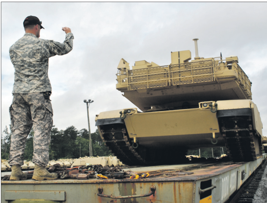
At left, Sgt. Joseph Howell, a Surface Maintenance Mechanic at MATES, acts as a ground guide for one of the new M1A2 SEP v2 Main Battle Tanks as the driver watches for hand signals during the offloading procedure.
