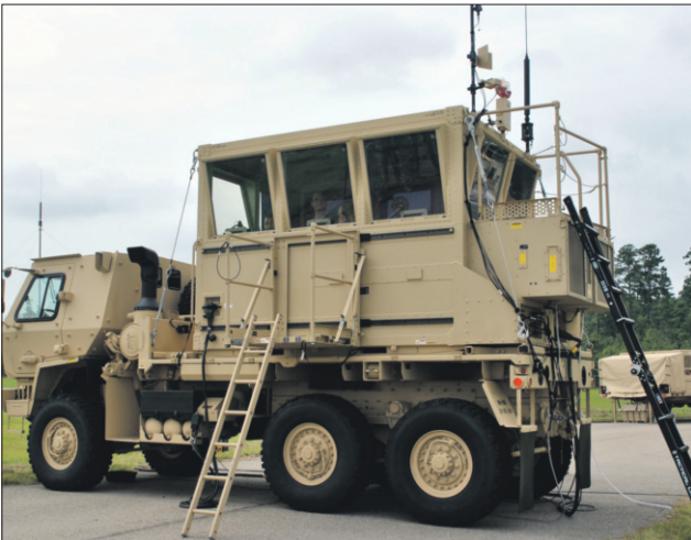
Air traffic controllers of the Mississippi National Guard's 2-185th Aviation Regiment man the unit's new AN/MSQ-135 Mobile Tower System during a media day held at Camp Shelby Joint Forces training Center July 24.
