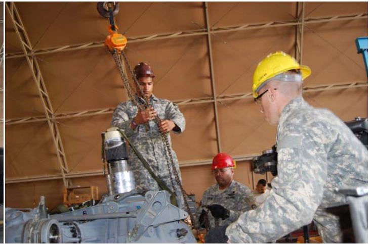
Pictured above: SPC Damon Lappe secures the main mod to the crane hoist with the properly rated chains and straps.
