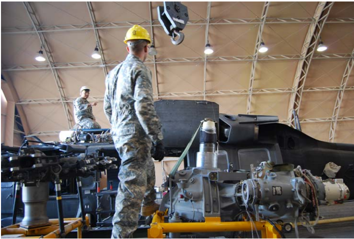
Pictured above: SPC Robert Wager communicates with Technical Inspector SGT Arturo Parra before hoisting the main transmission.
