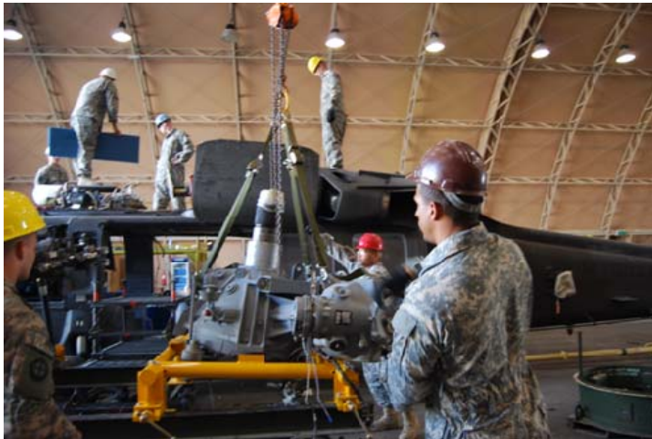
Pictured above: The dedicated members of the Airframe Repair Team prepares to lift the main UH-60 transmission module into place.
