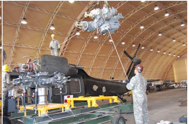
Pictured above: SPC Robert Wager (on top of the aircraft) and SPC Damon Lappe guide the main mod into place with precision and care.
