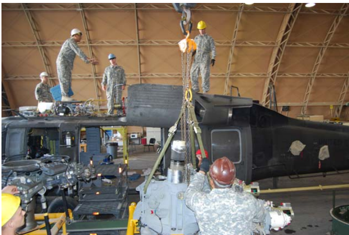
Pictured above: The dedicated members of the Airframe Repair Team prepares to lift the main UH-60 transmission module into place.
