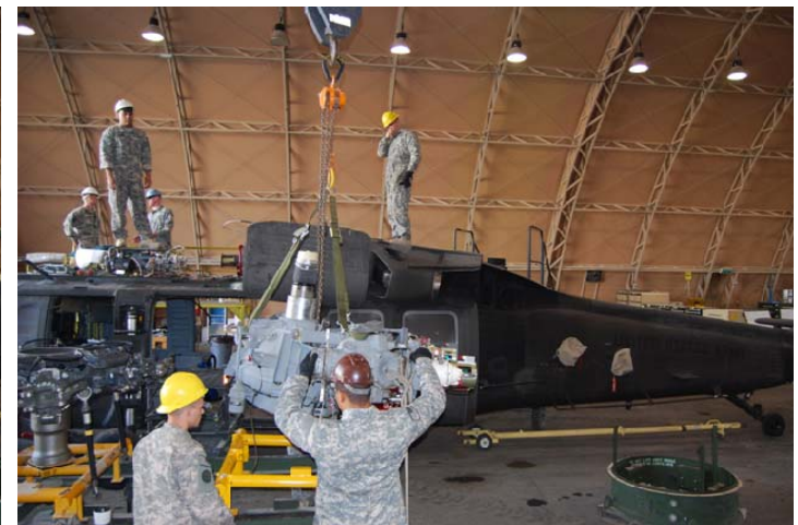
Pictured above: The dedicated members of the Airframe Repair Team prepares to lift the main UH-60 transmission module into place.
