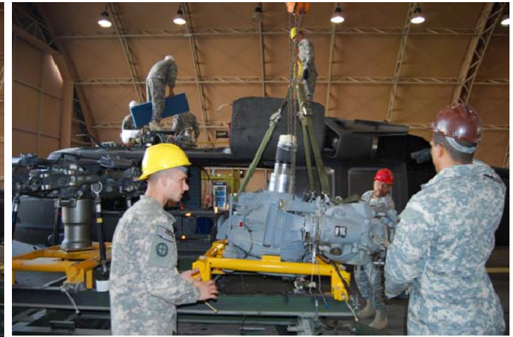
Pictured above: The dedicated members of the Airframe Repair Team prepares to lift the main UH-60 transmission module into place.
