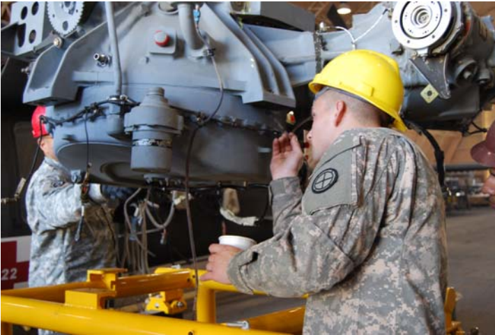
Pictured above: SPC Cody Smith applies Pro-Seal (an aircraft rated sealant) to the feet of the main transmission module before it is lifted into place.
