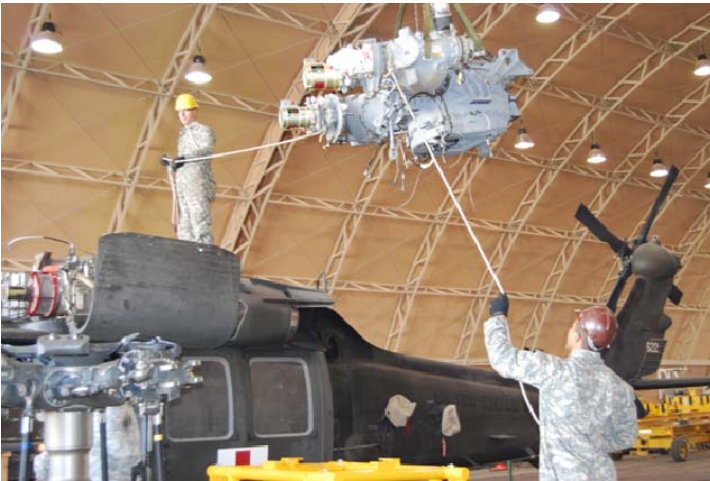
Pictured above: SPC Robert Wager (on top of the aircraft) and SPC Damon Lappe guide the main mod into place with precision and care.
