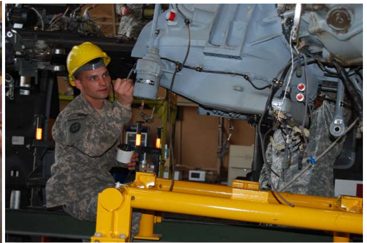
Pictured above: SPC Cody Smith applies Pro-Seal (an aircraft rated sealant) to the feet of the main transmission module before it is lifted into place.
