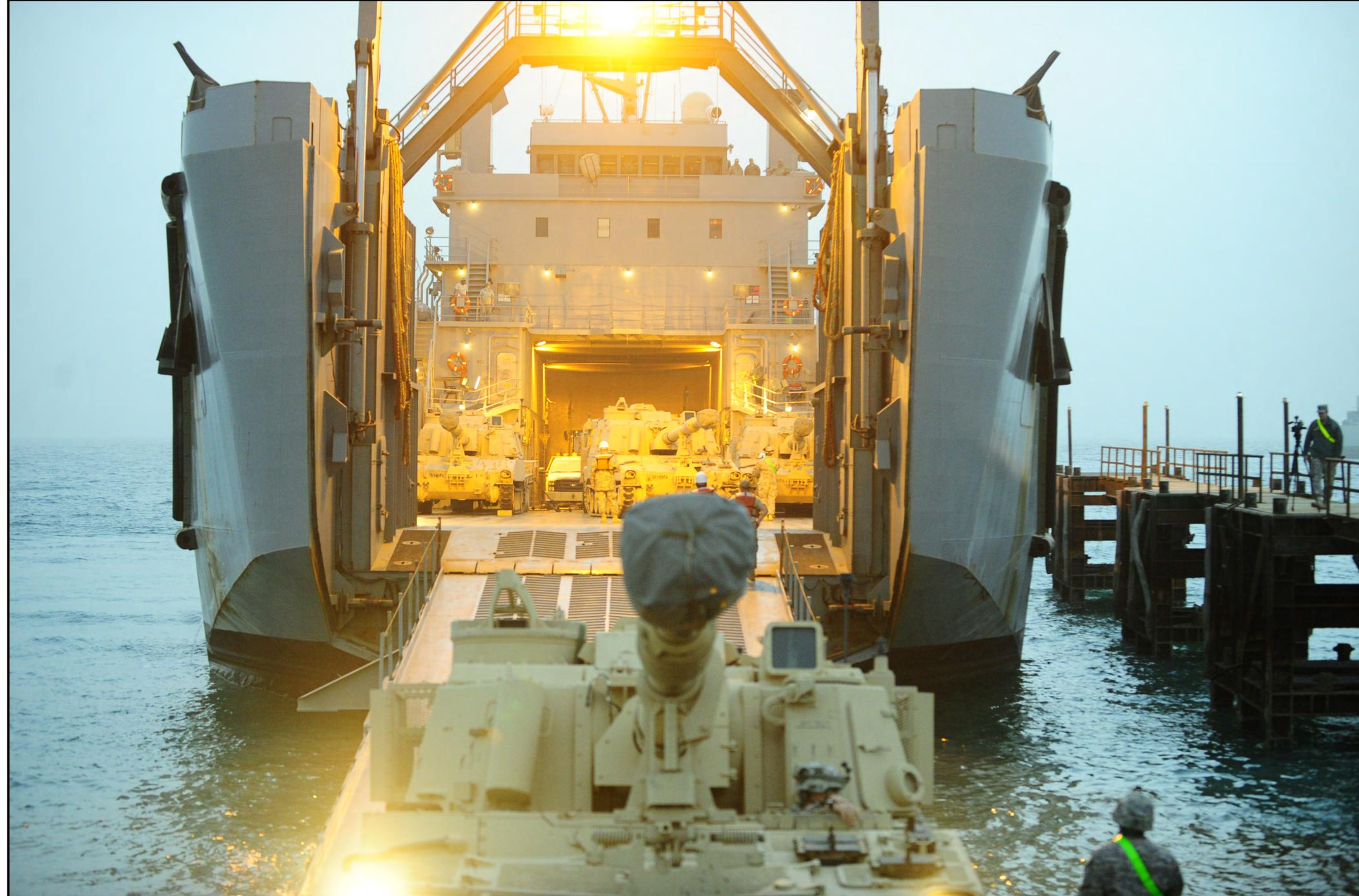
Chief Warrant Officer 2 Vernon Slaughter, vessel master of USAV Churubusco, explained that these vessels generally cruise at 12 knots even with six Bradleys, weighing over 150 tons, on board.
