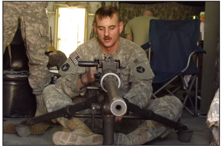
Cpl. Daniel Post, an Infantryman from Sauk Center, Minn., with Alpha Company, 1 st Combined Arms Battalion, 194 th Armor, instructs Expert Infantryman Badge candidates on how to properly set the head space and timing on the M2 .50cal machine gun. This training was conducted around the 1-194 CAB battalion area prior to sending Soldiers to Camp Buehring for additional training.
