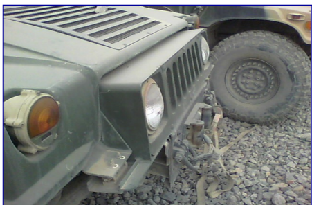
(1.1) The GEN III system bends the front face of the bumper plate affecting the structural integrity of the M1151
