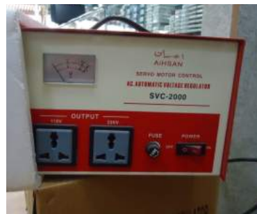
A non-UL or CE-approved transformer.
