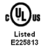
A counterfeit UL sticker. Note: "Listed" should be written in all capital letters. The product identity phrase is also missing.
