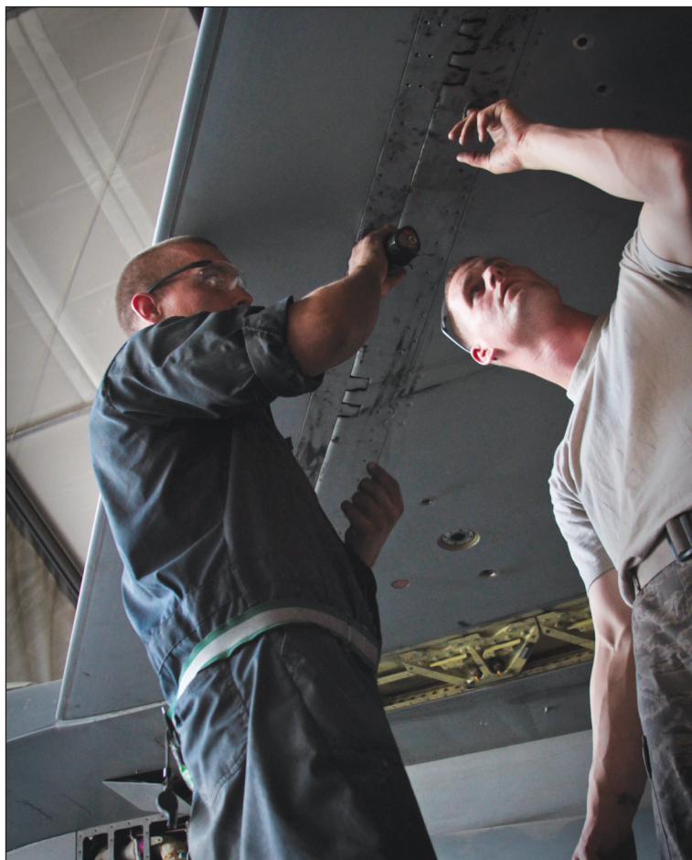
U.S. Air Force Airmen First Class Michael Jordan and Adam Sexton, 455th Expeditionary Aircraft Maintenance Squadron crew chiefs, secure rivets on the wing of an F-16C Fighting Falcon Oct. 4. (Photo by U.S. Air Force Tech. Sgt. Matt Hecht 455th PAO)
