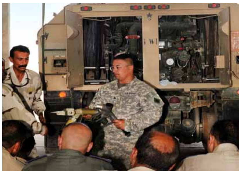
Sgt. Gilbert Britto of A Co., 640th ASB, shows a class of Iraqi Army personnel a fueling nozzle and how it connects to the fueling module on a Heavy Expanded Mobility Tactical Truck (HEMTT)
