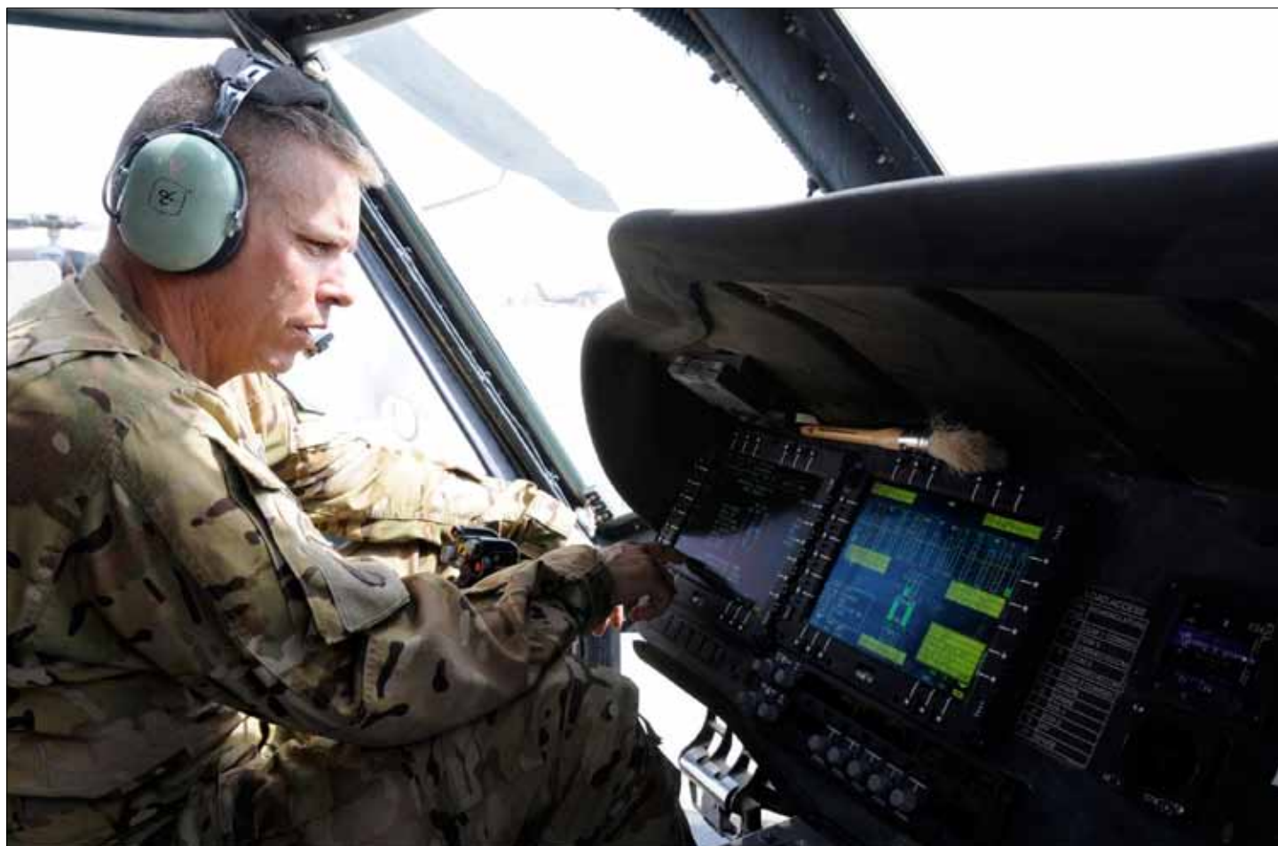
KANDAHAR AIRFIELD, Afghanistan (Aug. 24, 2011) - Chief Warrant Officer 4 Joel Sizelove, the production control officer in charge for Task Force Lift (7th Battalion, 101st Aviation Regiment), checks the readouts from the integrated vehicle health management system on a UH-60M Blackhawk to determine, among other things, track vibrations in the rotors. IVHMS ultimately saves maintainers hours or even days of work, and gets the aircraft and its crew back into the fight faster.
