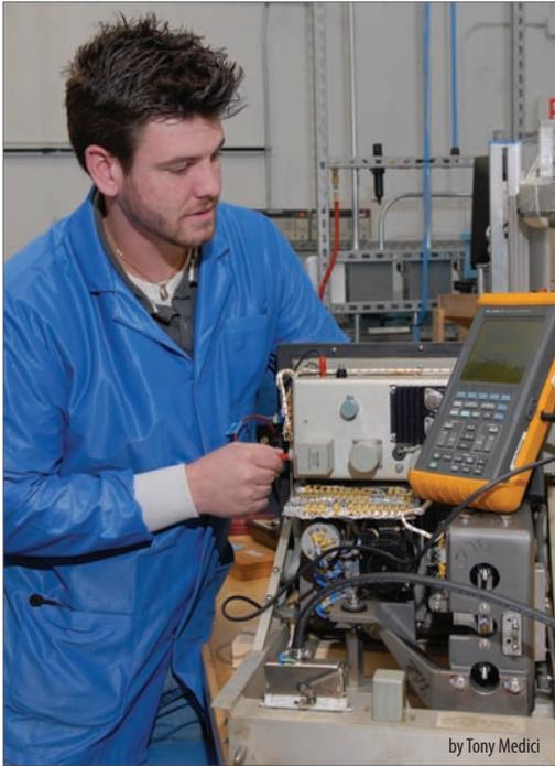
Electronics Mechanic, John Kostiak, checks input and output voltages from the main amplifier of a Depth Detector Type 2 at Tobyhanna Army Depot.
