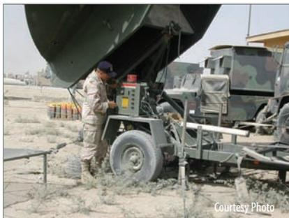
Larry Eberhardt aligns the LHGX (light weight high gain X-band antennae) 16 Foot antennae's junction box.
