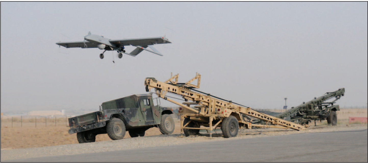
Above Left: Spc. Joshua Caldwell, a maintainer for the 1st Bde, 34th Inf. Div., BSTB, Minnesota National Guard, and a native of Redwing, Minn., checks the belt on a Unmanned Aerial Systems launcher during his preflight inspections at Forward Operating Base Sharana, Afghanistan Aug. 25.
