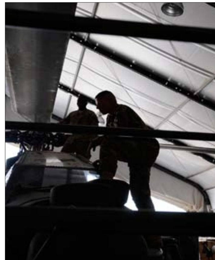
An AH60D Apache helicopter crew chief with Troop D, Task Force Palehorse (7th Squadron, 17th Cavalry Regiment), examines a blade to determine whether it needs repair or replacement here June 22.
