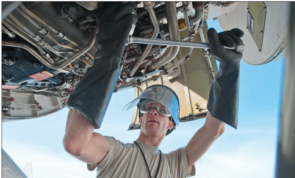
Senior Airman Benjamin Goldsmith, 517th Aircraft Maintenance Unit, replaces an oil filter on a C-17 Globemaster III, Wednesday. The C-17 was being prepared for the Air Mobility Command Rodeo. (U.S. Air Force photo/Senior Airman Christopher Gross)
