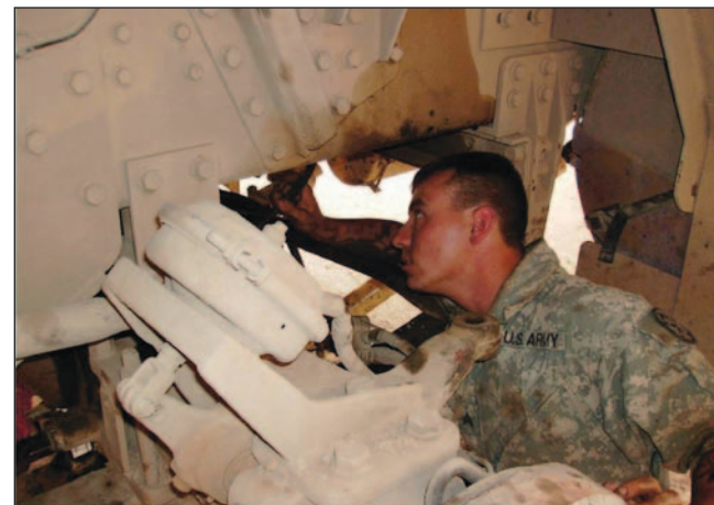
Sgt. Derrick T. Felch, a mechanic with the 68th Transportation Company, 749th Combat Sustainment Support Battalion, 4th Sustainment Brigade, 310th Expeditionary Sustainment Command, and a native of Bismarck, N.D., crouches under a truck as he removes the oil pan on Contingency Operating Base Adder, Iraq.
