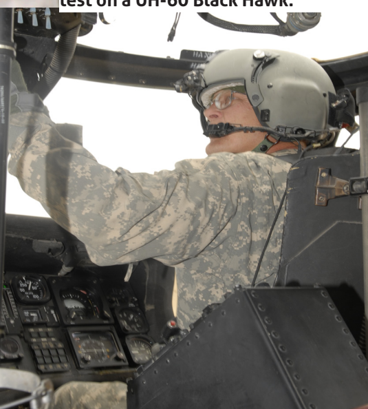
Chief Warrant Officer David Clark performs a maximum engine throttle test on a UH-60 Black Hawk.
