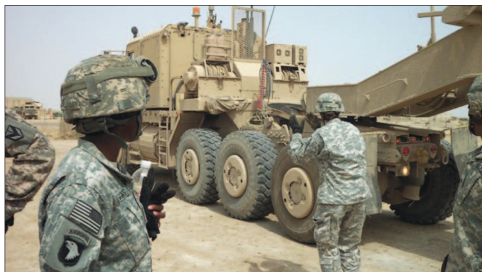
Spc. Jaclyn Bartlett, a heavy-wheeled vehicle operator with the 15th Transportation Company, 749th Combat Sustainment Support Battalion, 4th Sustainment Brigade, 310th Expeditionary Sustainment Command and a native of Norfolk, Va., demonstrates ground guiding a heavy-equipment transport vehicle to its trailer at Contingency Operating Base Adder, Iraq.
