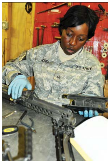
Sgt. Natasha King, a small-arms weapons repairer and native of Fort Pierce, Fla., disassembles an M249 Squad Automatic Weapon in order to properly replace the rear sight of the weapon.
