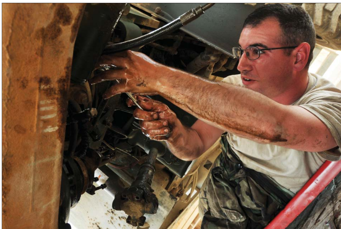
Spc. Christopher Smith, a native of Walnut Cove, N.C. and a construction equipment repairer for the 632nd Maintenance Company, 749th Combat Sustainment Support Battalion, 4th Sustainment Brigade, 310th Expeditionary Sustainment Command, works to replace the hydraulic hoses on a 10K Atlas Forklift. Smith and his fellow "Outlaws" may be on their way out the door, but their mission effectiveness will leave a lasting mark on operations here.
