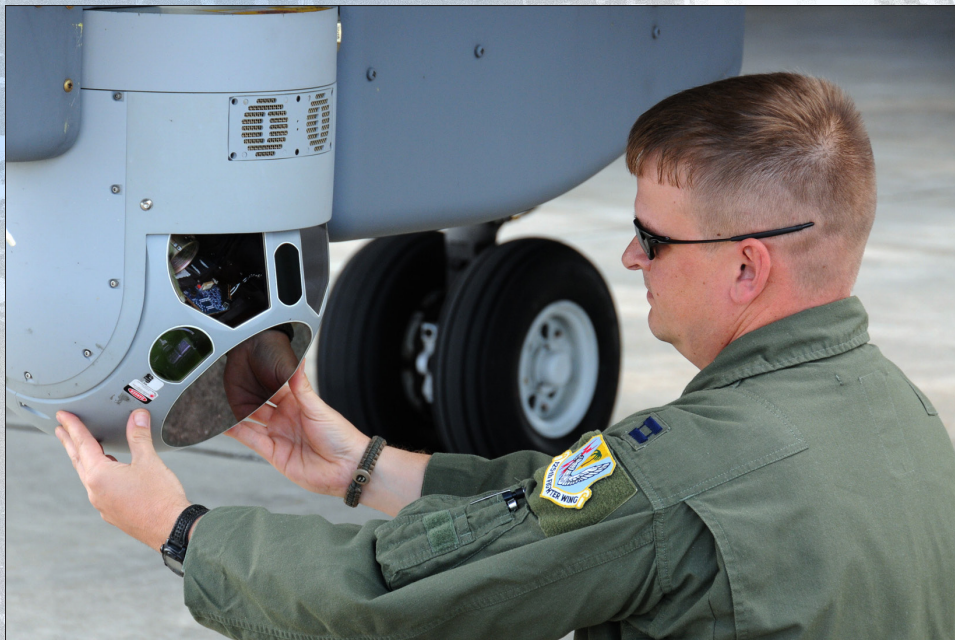
An RC-26B mission systems operator from the Florida Air National Guard, 125th Fighter Wing, based out of Jacksonville, Fla., conducted preflight inspection of the optics in the sensor turret before a training mission off the coast of Jacksonville, Fla., Jan. 22. The RC-26B is equipped with full motion streaming video, laser range finder, laser illuminator and other systems capabilities which enables real-time monitoring during critical law enforcement surveillance missions.
