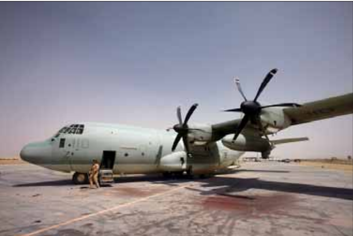
STAFF SGT. CHRISTOPHER FLURRY Cpl. Jessica M. Egan, a crew chief with Marine Aerial Refueler Transport Squadron 352, performs a preflight inspection on the Harvest Hawk-equipped KC-130J at Camp Dwyer, Afghanistan, March 25. The one-of-a-kind Harvest Hawk system includes a version of the target sight sensor used on the AH-1Z Super Cobra attack helicopter as well as a complement of four AGM-114 Hellfire and 10 Griffin missiles.
