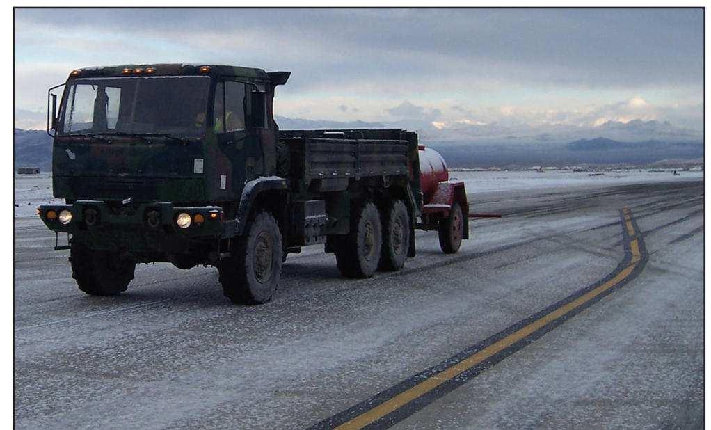
(Top) A Soldier from Company E, Task Force Knighthawk, 10th Combat Aviation Brigade, 10th Mountain Division, demonstrates how de-icing fluid flows through the holes of a fabricated pipe before de-icing the runway at Forward Operating Base Shank. Soldiers of Co. E, TF Knighthawk, constructed the de-icer from an Army water trailer this winter to remove ice from the runway at the FOB. (Photo by U.S. Army Sgt. Janell Emerson, Task Force Knighthawk) (Bottom) The runway at Forward Operating Base Shank is de-iced with a collaboration made with an Army water trailer by Soldiers of Company E, Task Force Knighthawk, 10th Combat Aviation Brigade, 10th Mountain Division. (Photo courtesy of David Guarino)
