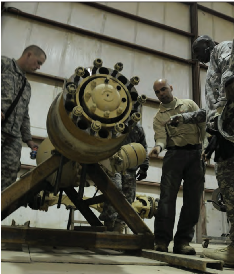
Anthony Weathers shows Soldiers the brake chamber on the axle of an MRAP during their familiarization training on Camp Victory, Jan 5.
