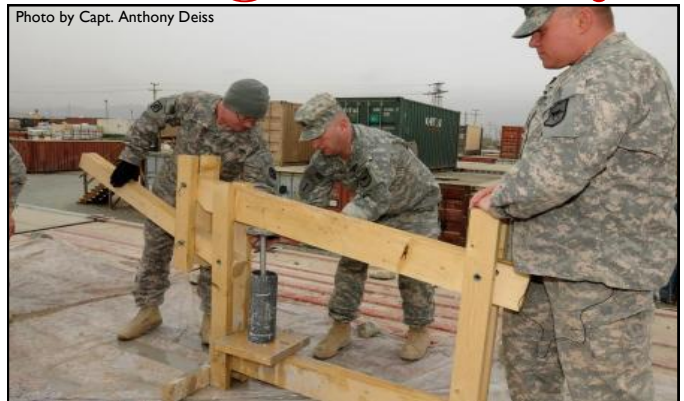
Photo by Capt. Anthony Deiss Chief Warrant Officer 2 Kent Frye, left, 902nd Engineer Company, and Sgt. John Shyne, 196th Maneuver Enhancement Brigade, center, make a “fuel donut” using a press made from scrap lumber as Capt. Robert Small, 196th, provides stability to the press Jan. 29 at Camp Phoenix in Kabul, Afghanistan.
