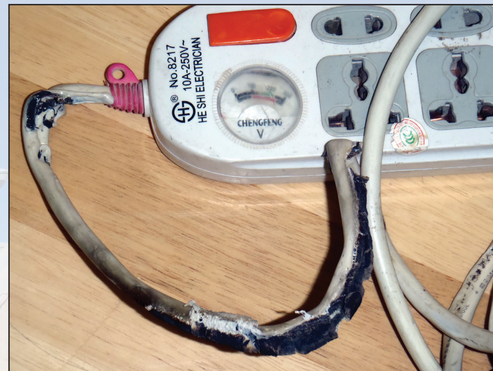
This non-UL/CE power strip/surge protector was overloaded and burned causing significant damage.
