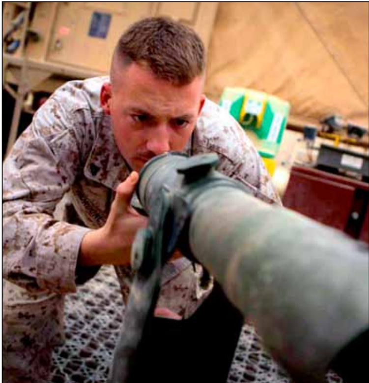
CAMP DWYER, Afghanistan-Cpl. Joseph Nordone, 21, electro-optical ordnance repairman, Support Company, Combat Logistics Battalion 3, 1st Marine Logistics Group (Forward), inspects a M1A1 Collimator aboard Camp Dwyer, Afghanistan, Jan. 10. The Collimator is a device used to assist artillery units in maintaining accurate fires when firing missions. Cpl. Daniel H. Woodall/1st Marine Logistics Group (FWD)
