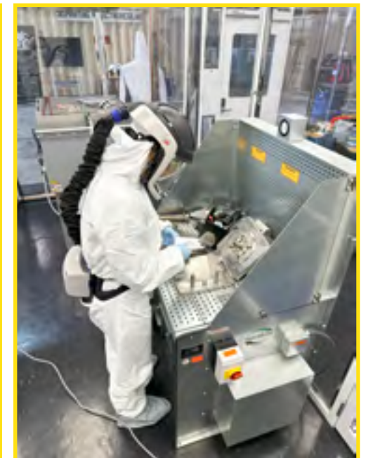
NAVFAC EXWC personnel train on a Concept Laser M2 Direct Metal Laser Melting (DMLM) machine to accelerate NAVFAC EXWC’s prototyping capabilities, at the FATHOMWERX innovation lab at the Port of Hueneme.
