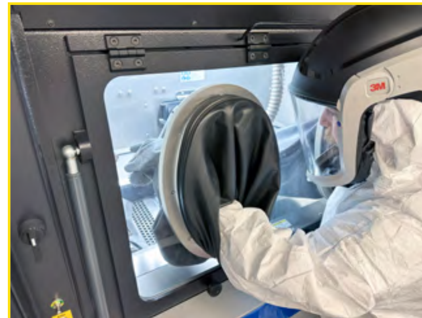
NAVFAC EXWC personnel train on a Concept Laser M2 Direct Metal Laser Melting (DMLM) machine to accelerate NAVFAC EXWC’s prototyping capabilities, at the FATHOMWERX innovation lab at the Port of Hueneme.
