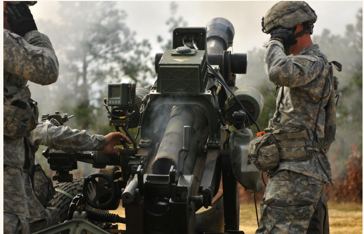
Paratroopers of the 2nd Battalion, 319th Airborne Field Artillery Regiment, 2nd Brigade Combat Team, 82nd Airborne Division, fire a newly fielded M119A3 howitzer on Fort Bragg, NC. The 2-319th AFAR became the second artillery battalion in the 82nd Abn. Div. to receive new howitzers equipped with a digital fire control system that allows artillery crews to emplace the gun and begin firing rounds in less than two minutes. (Photo by Staff Sgt. Jason Hull)
