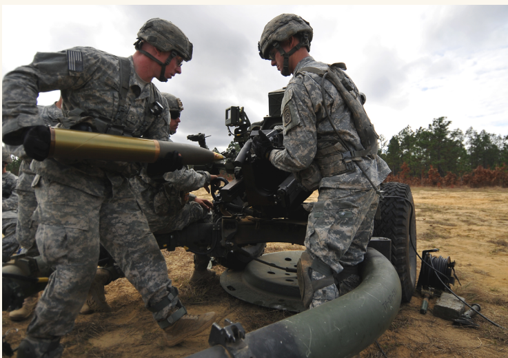
Paratroopers of the 2nd Battalion, 319th Airborne Field Artillery Regiment, 2nd Brigade Combat Team, 82nd Airborne Division, load a 105 mm artillery round into a newly fielded M119A3 howitzer on Fort Bragg, NC. The 2-319th AFAR became the second artillery battalion in the 82nd Abn. Div. to receive new howitzers equipped with a digital fire control system that allows artillery crews to emplace the gun and begin firing rounds in less than two minutes. (Photo by Staff Sgt. Jason Hull)
