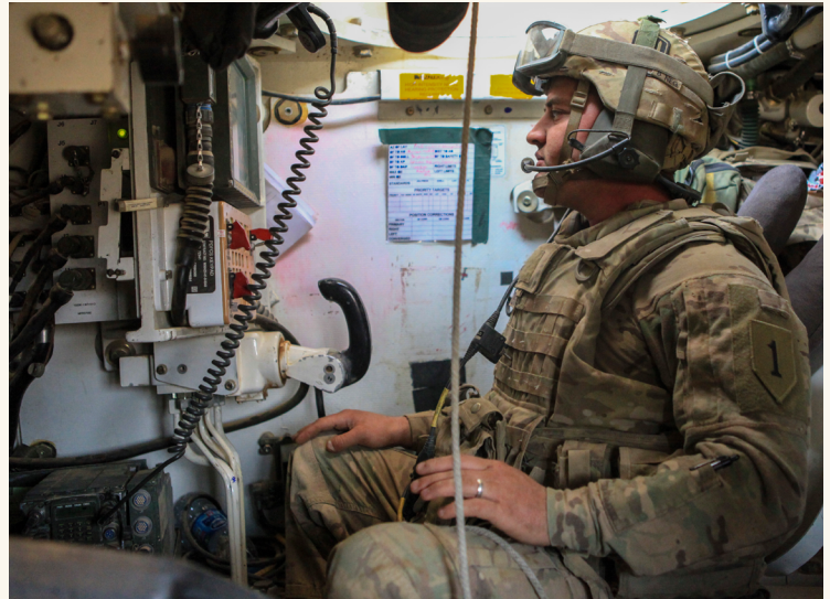
U.S. Army Staff Sgt. Boett Stovall, with the B-Battery, 1st Infantry Battalion, 7th Field Artillery Regiment, 1st Infantry Division, reads a Paladin Digital Fire Control System in a Paladin M109 Alpha-6 Howitzer to provide a digital link to the fire support network for calls-for-fire and mission data during exercise Eager Lion 2016, at Al Zarqa, Jordan (U.S. Army photo by Spc. Kevin Kim/ Released)
