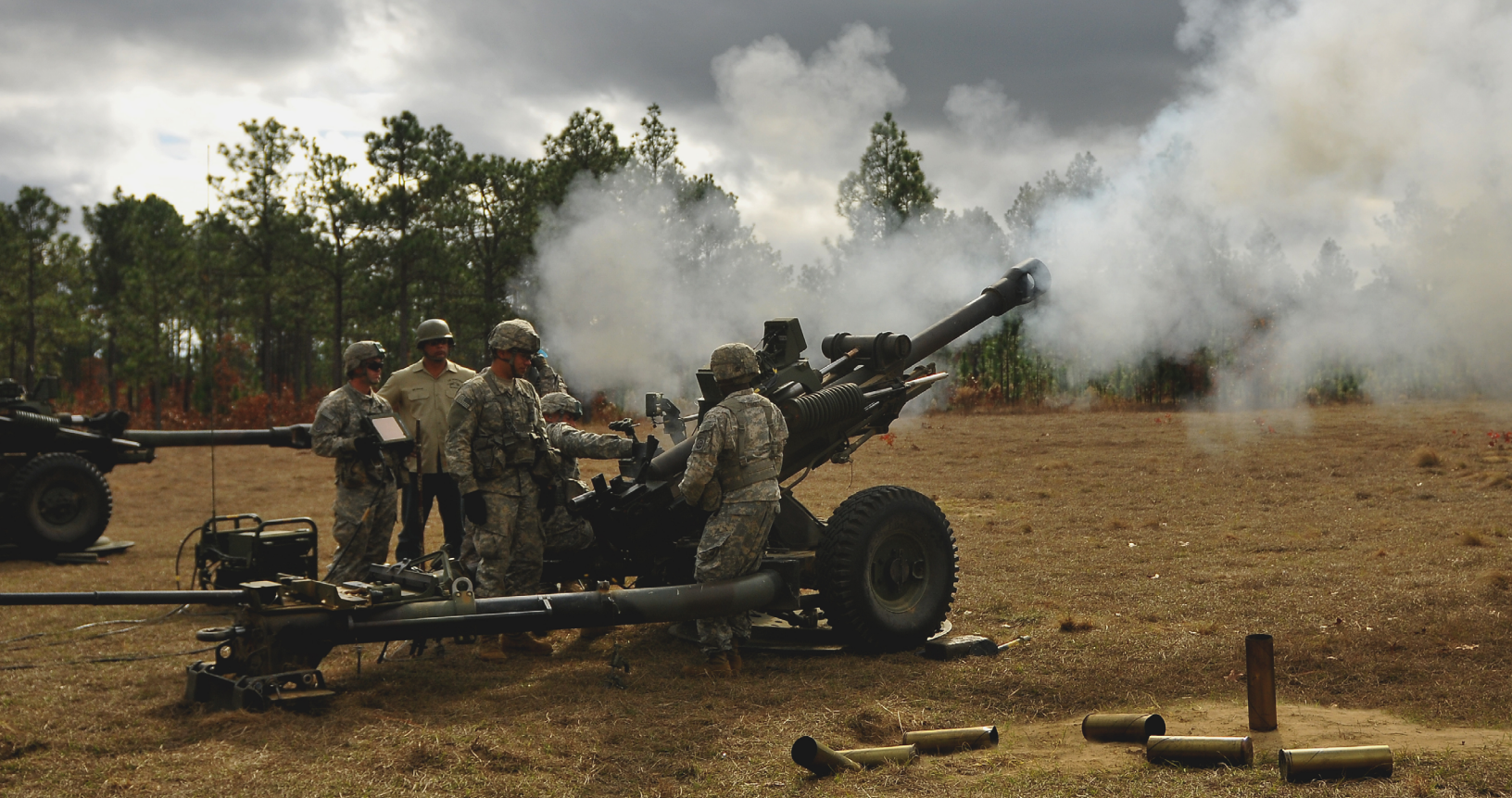
Paratroopers of the 2nd Battalion, 319th Airborne Field Artillery Regiment, 2nd Brigade Combat Team, 82nd Airborne Division, fire newly fielded M119A3 howitzers on Fort Bragg, N.C., Nov. 22. The 2-319th AFAR became the second artillery battalion in the 82nd Abn. Div. to receive new howitzers equipped with a digital fire control system that contains software similar to the Army's M777A2 howitzers. (Photo by Staff Sgt. Jason Hull)
