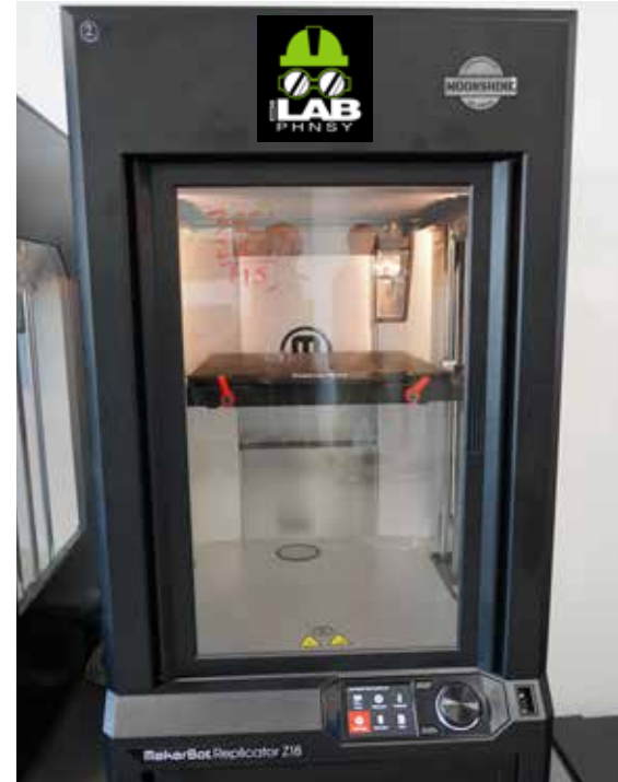
MakerBot Replicator Z18, one of the different additive manufacturing printers that is located in the iLAB. Capable of printing PLA Filament with a build volume of 30"L X 30.5"W X 45.7"H.
