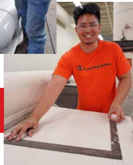
Shop 57 Insulator Apprentice Lawrence Raze lays out patterns for insulation fabrication in support of USS Hawaii (SSN 776).
