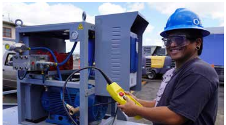
Shop 06 Production Machinery Maintenance Apprentice Elyjah Sumile operates a water-blast machine to support blasting ships hulls and piping systems.
