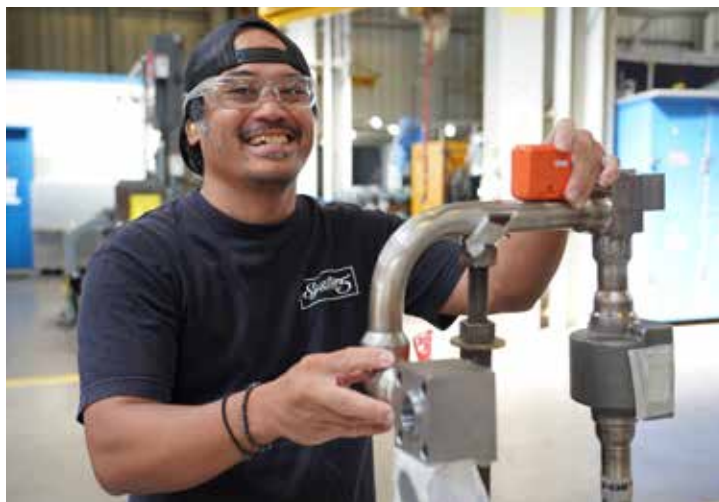
Shop 56 Work Leader Elias Cabebe is checking piping alignment utilizing a digital angle finder.
