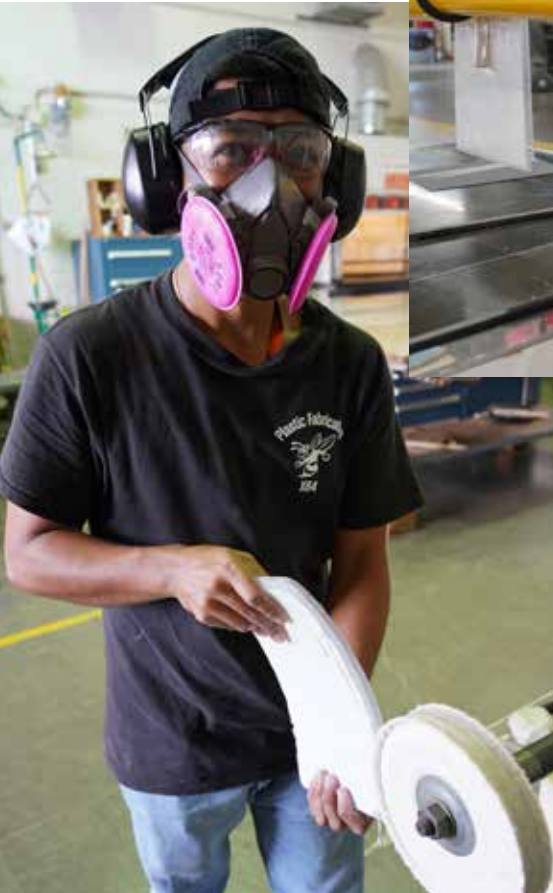
Shop 64PF Plastic Fabricator Mechanic Jeffrey Soriano buffs a piece of plexiglass to fit up in the crew's mess on USS Missouri (SSN 780).
