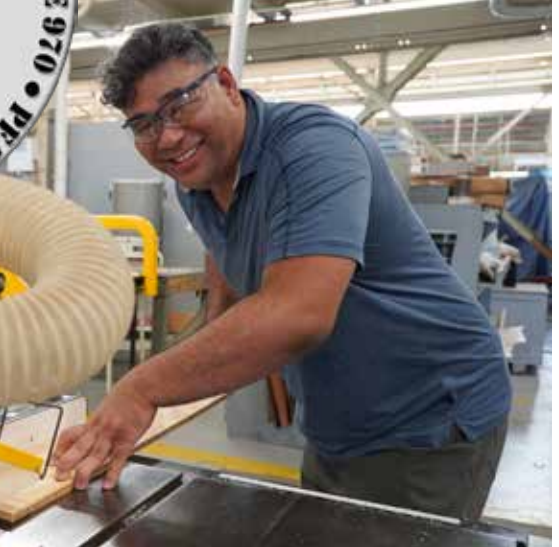
Shop 64PF Plastic Fabricator Mechanic Lee Nouchi performs a rip cut on a piece of plywood which will be used to build cabinets for various dry dock projects.
