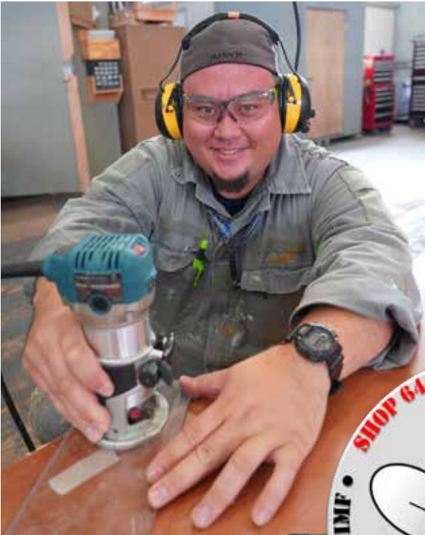
Shop 64PF Plastic Fabricator Mechanic Blaine Hook utilizes a router to finish the edge of a wooden table top that will be used on the USS Hawaii (SSN 776) project.
