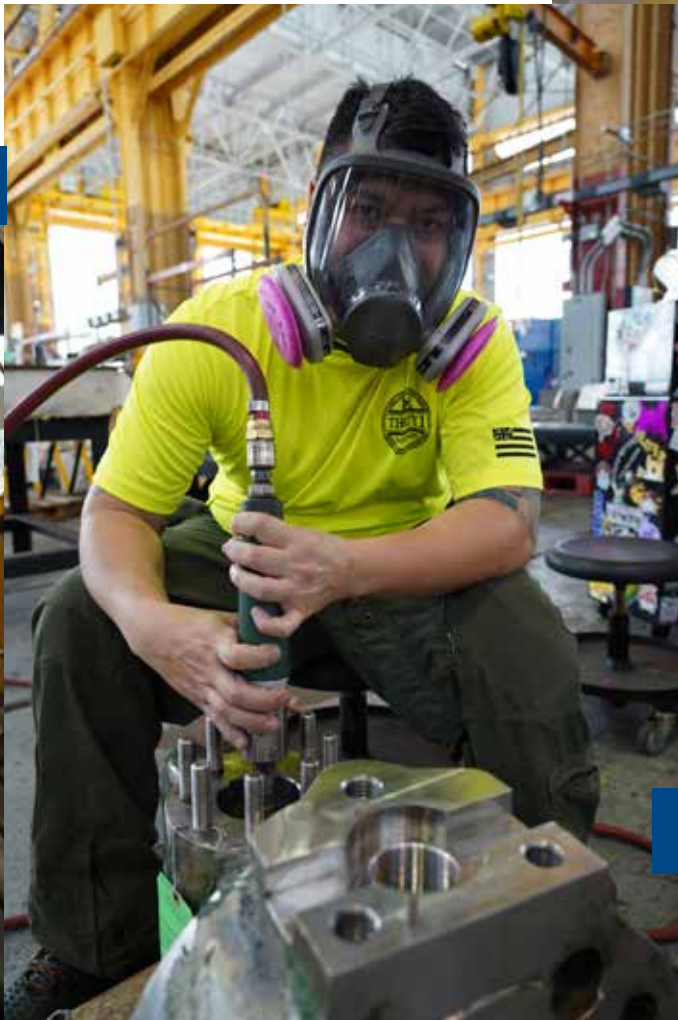
Shop 31 Machinist Mechanic Bronson Tabios cleans the internals of a valve body prior to inspections.
