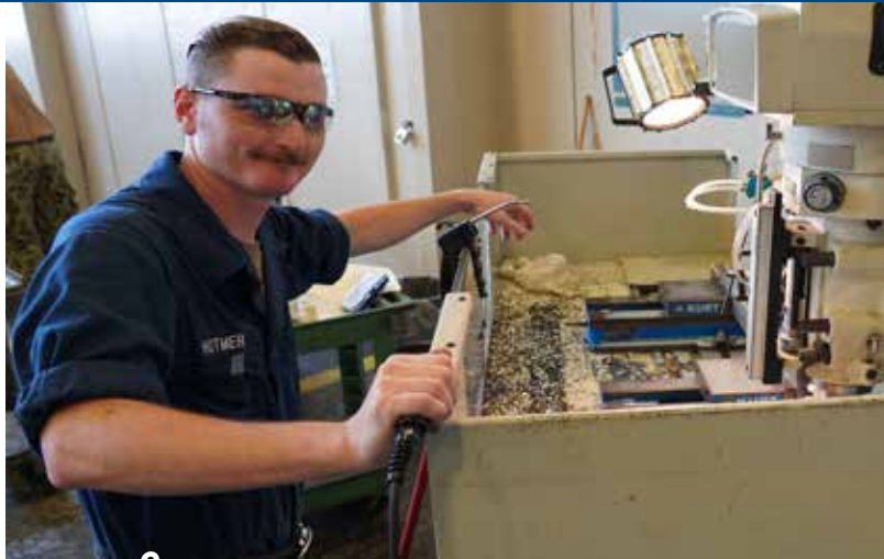
Shop 31 Machinist Repairman 1st Class Frank Hotmer operates a CNC (computerized numerical control) mill.
