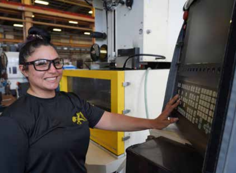
Shop 31 Machinist Apprentice Amelinda Kim programs a wire electrical discharge machine.
