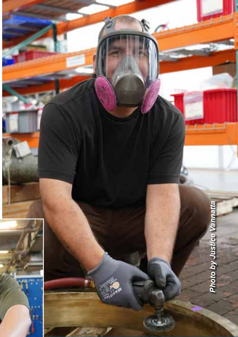
Shop 38 Marine Machinery Mechanic Aaron Greer cleans a Virginia-class submarine eccentric bearing in preparations for inspections and measurements.
