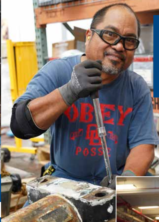
Shop 38 Marine Machinery Repairer Derwin Villegas is in the process of disassembling a vertical launch system hatch assembly.
