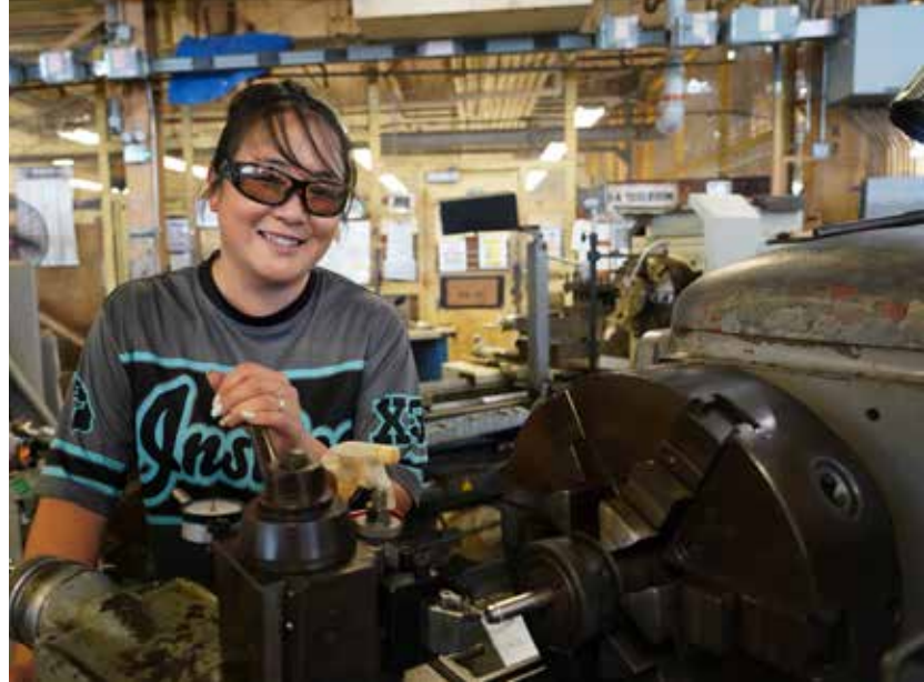
Shop 31 Machinist Apprentice Shana Hinokuma turns down metal barstock on a manual lathe.
