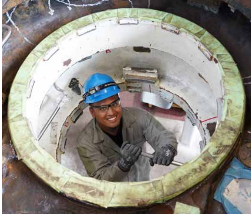
Shop 38 Marine Machinery Helper Anthony Kaulili preps a logistics plug trunk during resource repairs.
