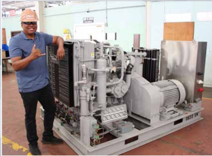
Code 987 Reliability Engineer Sterling Halmas is standing next to Shop 06's brand new Universal Highpack Compressor. It is an industrial air compressor that services and maintains high air pressure for tanks aboard the ships.
