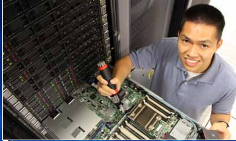
C109.11 System Administrator Victor Loui replaces server blade fans in the server farm to ensure proper cooling and fault tolerance.
