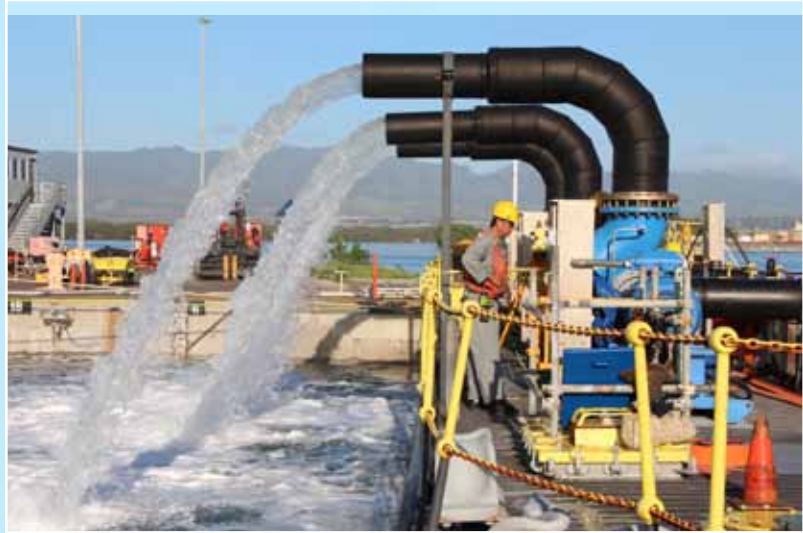
Shop 99 Dry Dock Industrial Equipment SME, Sean Ho operates the three Super Flood Pumps on DD3 Caisson during the Chicago Docking Evolution.
