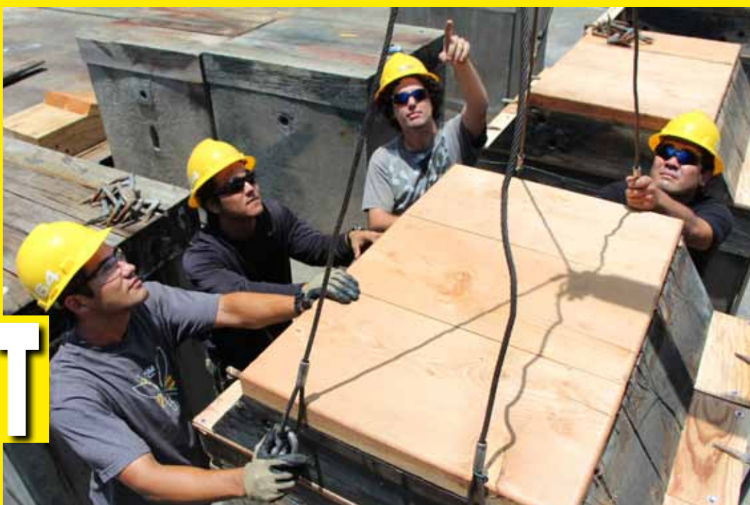
Shop 64 Shipwright Mechanics Justin Gideon, Rance David and Ryan Uno position a keel block for an upcoming docking with Shop 64 Shipwright Supervisor Renny Muraoka.
