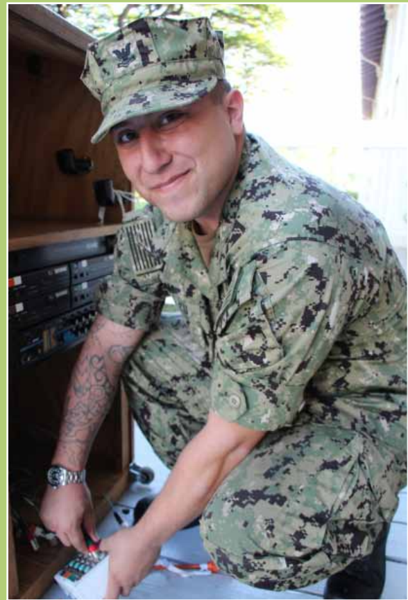
ETR2 David Martinez wires up the podium to the mixing console using an interconnecting audio box.
