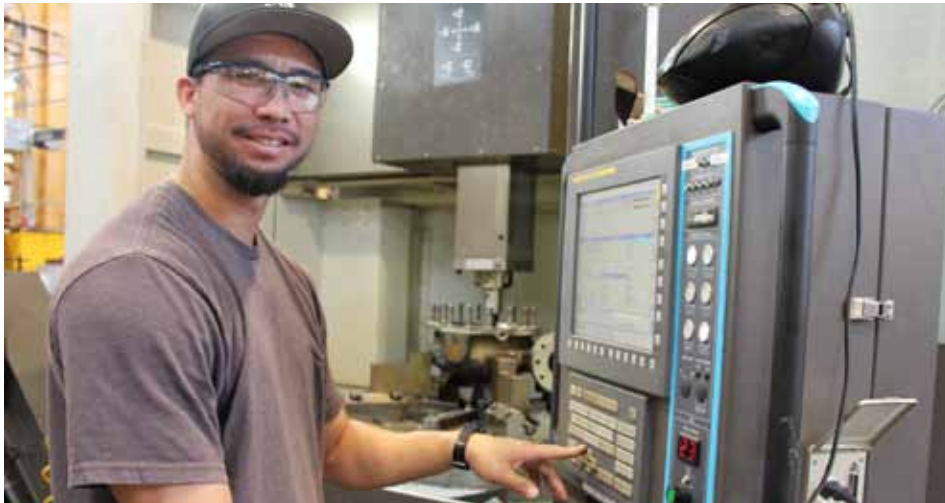
Code 930 Marine Machinist Mechanic Spenser McCready performs a multi-axis cut on a state-of-the-art, Hanlock vertical turret lathe to manufacture an Auxillary Sea Water Pump 2, in support of USS North Carolina SSN-777.
