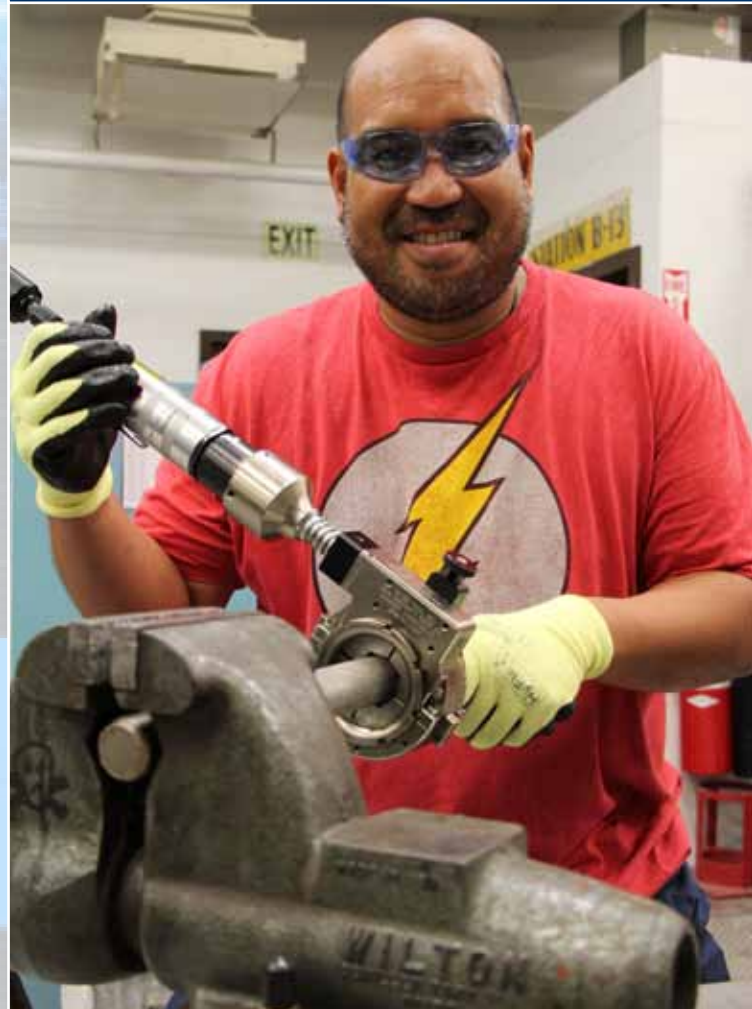
Shop 38 ST (Special Tools) Nuclear Marine Machinist Mechanic Daryl Dikilato secures a low profile clamshell split frame pipe lathe on to a one-inch pipe stock in support of USS Jefferson City (SSN - 759.)
