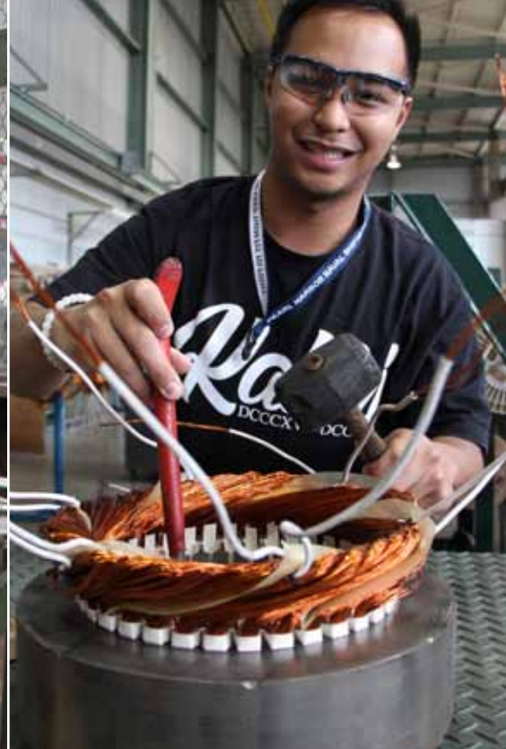
Shop 51 first year Electrical Apprentice Micah Rabanal is pounding copper wiring into place, while rewinding coils on a vent fan stator.
