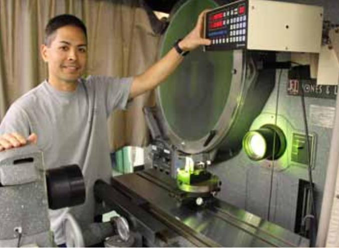
Code 950 Electronics Mechanic Dayven Higa is pictured in Shop 67 Physical-Dimensional Lab. He is measuring items with light on the Optical Comparator. This allows him to get a gauge of thickness for odd shaped parts.
