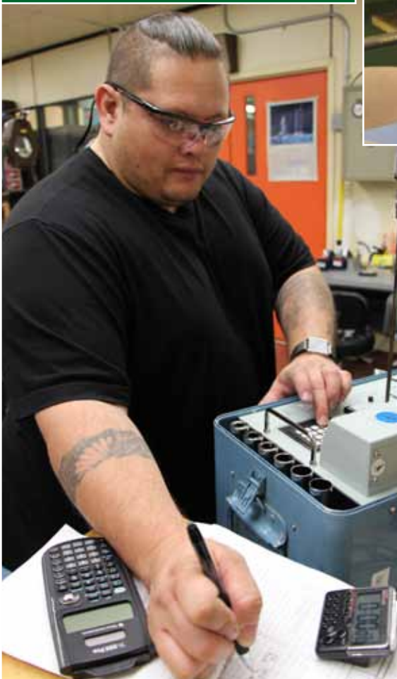
Code 950 Electrical Mechanic, Deayonne Barquis is issuing an annual calibration of the Temperature Calibration device. The component is used to accurately measure temperature readings.
