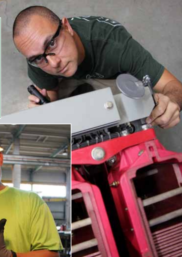
Shop 51 Breaker Supervisor, Robert "Uila" Barnett does a final inspection on a diesel generator breaker that will be installed on USS Greenville (SSN - 772.)
