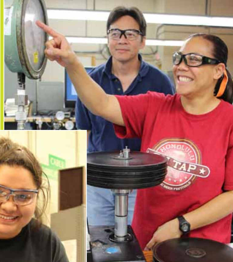
Shop 52 Mechanical Lab Engineer Aaron Young oversees first year Calibrations Apprentice Lavina Barbadillo as she takes readings on the Dead Weight Tester Laboratory Pressure Standard to make sure it reads the perfect nominal 400PSI.
