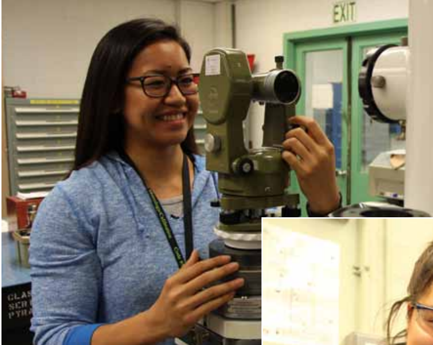
Shop 67 first year Calibrations Apprentice Noelani Mikami is looking through a Kern Theodolite. It is a precision instrument used for measuring angles in the horizontal and vertical planes. These measurements will be used for electrical systems on the USS Jefferson City (SSN - 759.)
