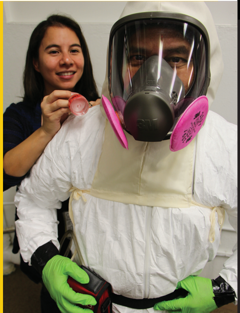
Code 106.11 Industrial Hygienists Kimberly Kalama and Code 106.11 Industrial Hygienists Andrew Cruz demonstrate workplace monitoring. An air monitoring pump and cassette is used to sample for occupational exposure to heavy metals such as lead, arsenic, cadmium, chromate and beryllium.
