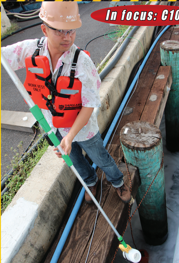
Code 106.31 Environmental Engineer Ernesto "Sto" Aban is verifying a dry dock permit compliance by sampling the water quality at the dry dock outfall at Gan Dock 4.
