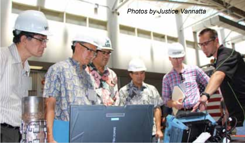
Code 138.3 Ultrasonic Test Examiner Cory Arthur demonstrates the ultrasonics of welds on the Phased Array machine. It is an advanced method of ultrasonic testing that has applications in imaging and industrial nondestructive testing.
