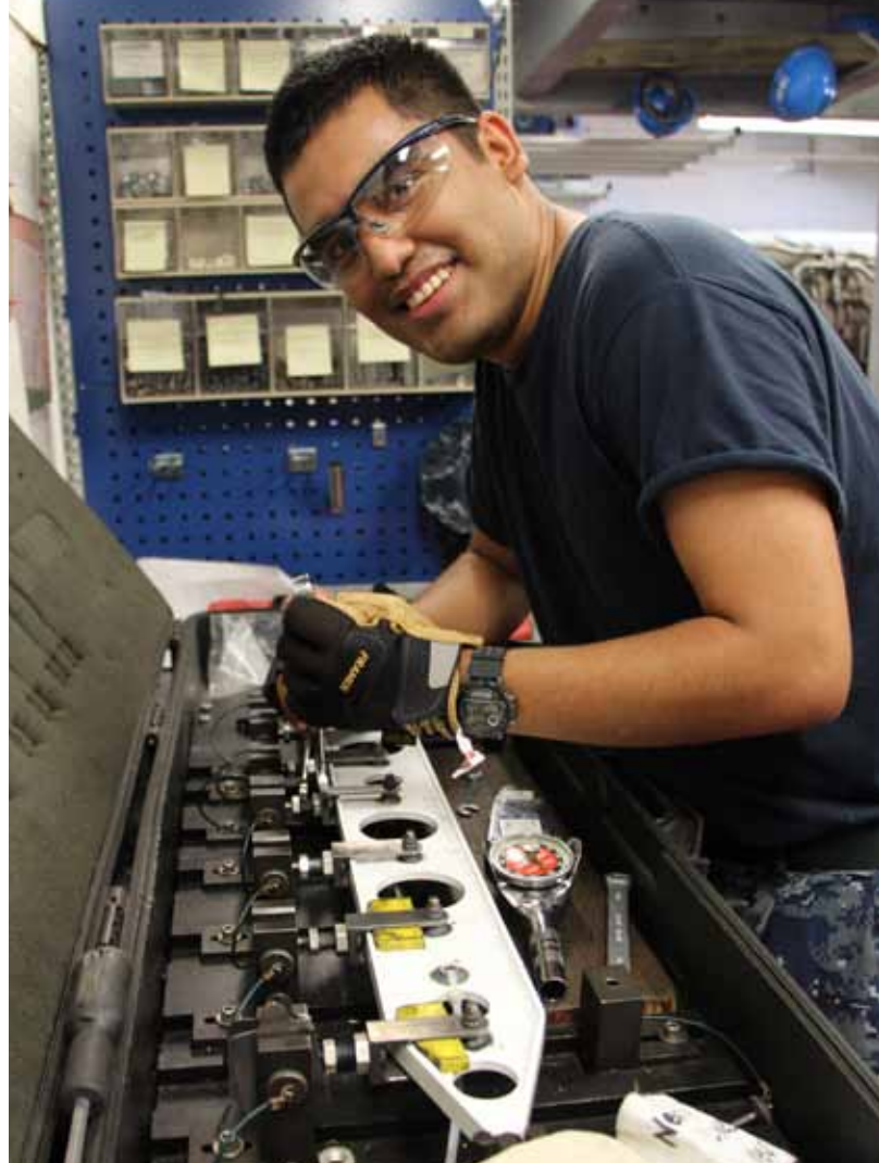
Code 930 GSM2 Neri repairs the VSV Arm Rigging. The VSV Arm is attached to the gas turbine engine to prevent the gas generator from stalling.
