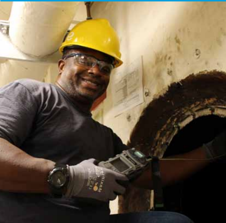
Code 990 Gas Free Monitor Franklin Reis performs a gas free test on a confined space ensuring proper air quality to allow workers to enter and do work.
