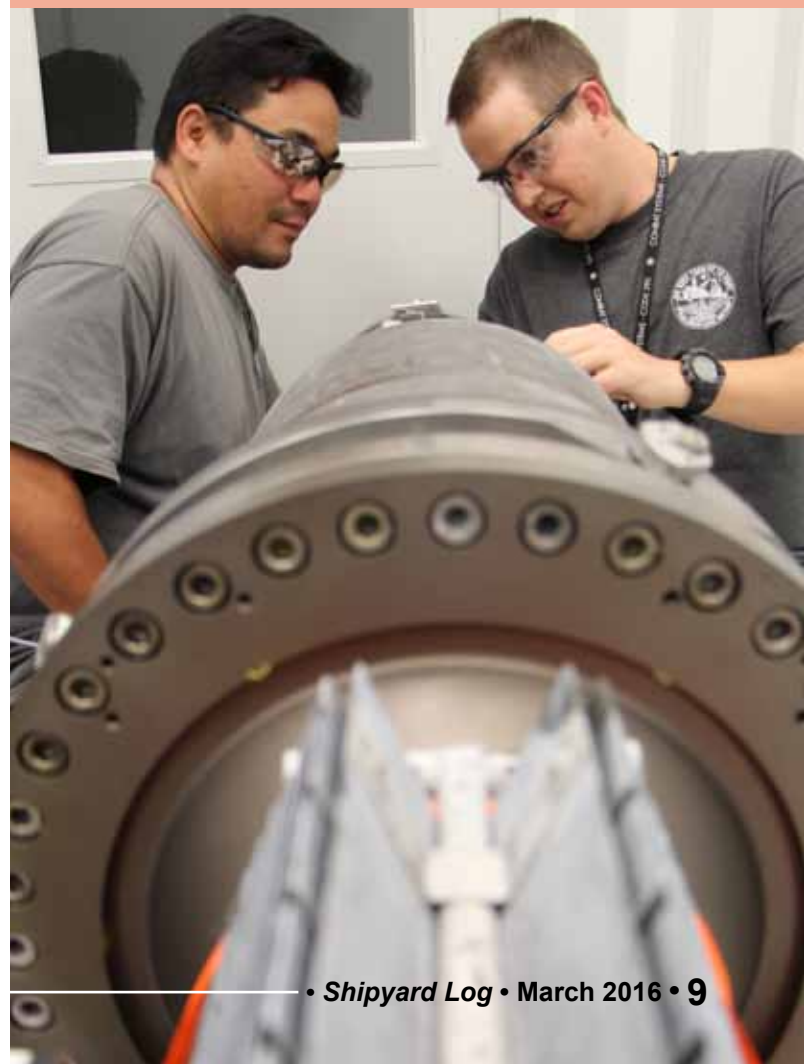
Code 290 Combat Systems Engineer Nick Fisher troubleshoots a photonics mast in the Shipyard's Photonics Laboratory in support of USS Mississippi (SSN 782) emergent work with Shop 67 Electrical Work Leader Mike Won.
