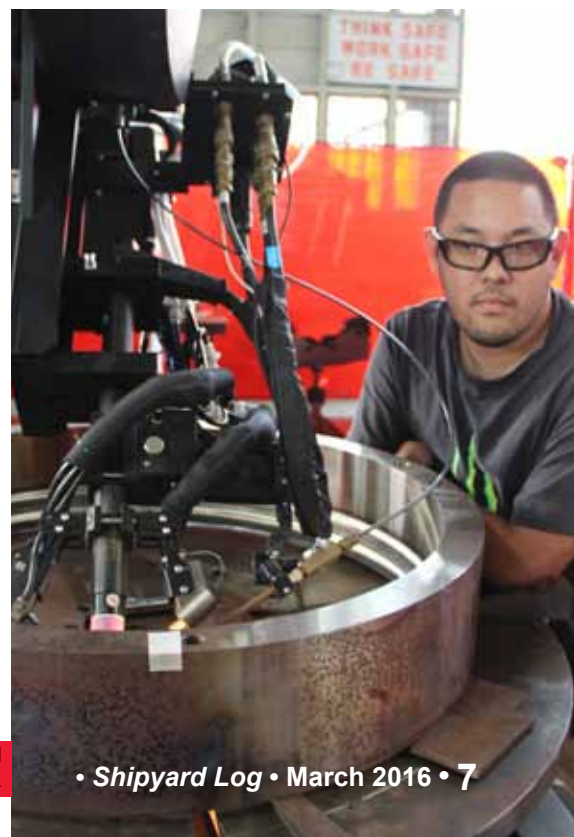
Shop 26 Welder Work Leader Kyle Toyota performs clad welding using their AMET automated GTAW welding machine.
