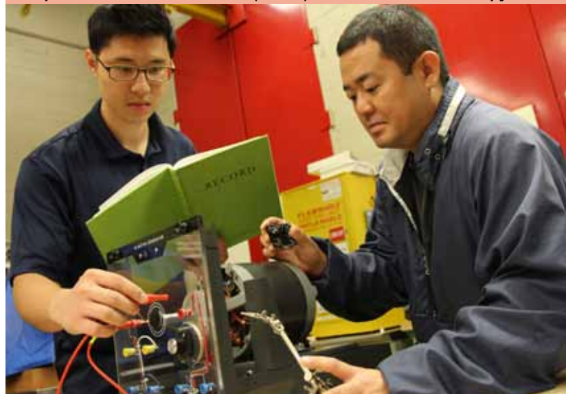
Code 270 electrical engineer Dewei Liu helps Shop 51 electrical mechanic Mike Higa assemble the Direct Current (DC) motor sparking tool. The DC motor sparking tool has the capability to identify and correct sparking issues automatically on DC motors, resulting in decreased Ships Service Motor Generator (SSMG) maintenance for the Shipyard.
