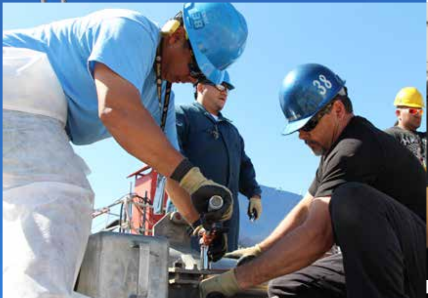
Code 930 Marine Machinist Mechanics Stuart Leong, Ron Gideon and Darren Agena secure metal clamps onto the Periscope in preparation of a crane lift, hoisting it onto the USS Asheville (SSN - 758.)
