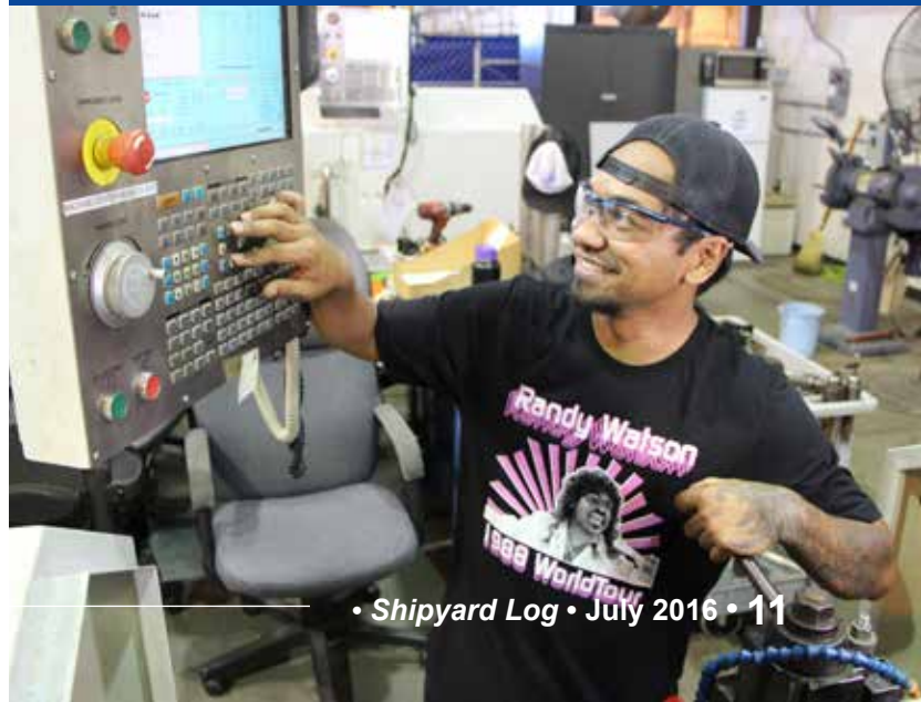
Shop 31 Machinist Work Leader Jacob Spencer operates a CNC Lathe, producing parts and cutting operation time by 50%, compared to the older processes in the past. Shop 31 supports all Submarines in the Intermediate Maintenance Facility.
