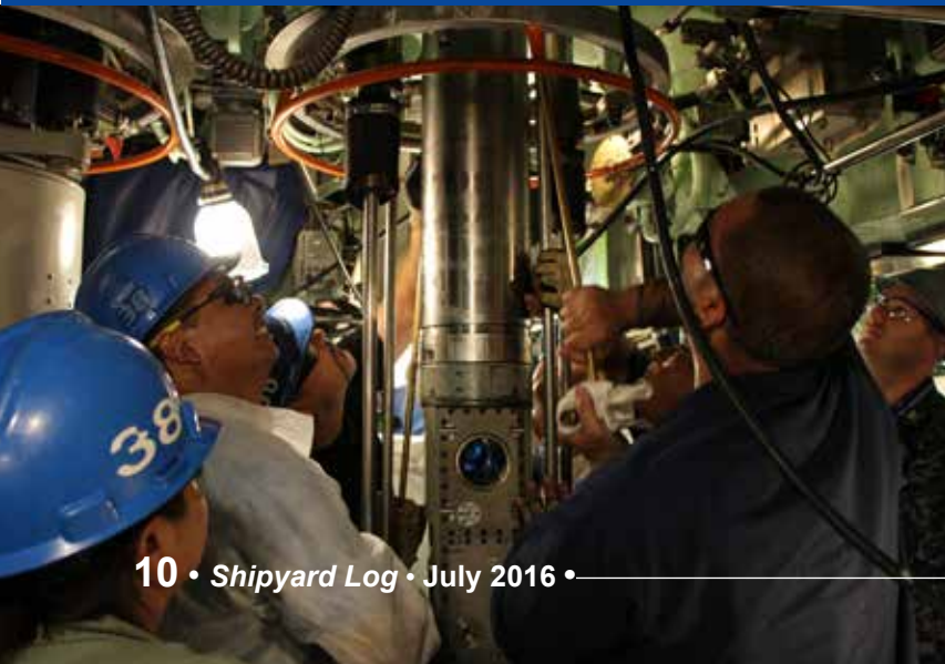
Code 930 Marine Machinist Mechanics Tiffany Makiya, Stuart Leong, Kala Akiona, and Ron Gideon install the Hull Gland for Periscope #1 on board the USS Asheville (SSN - 758.)
