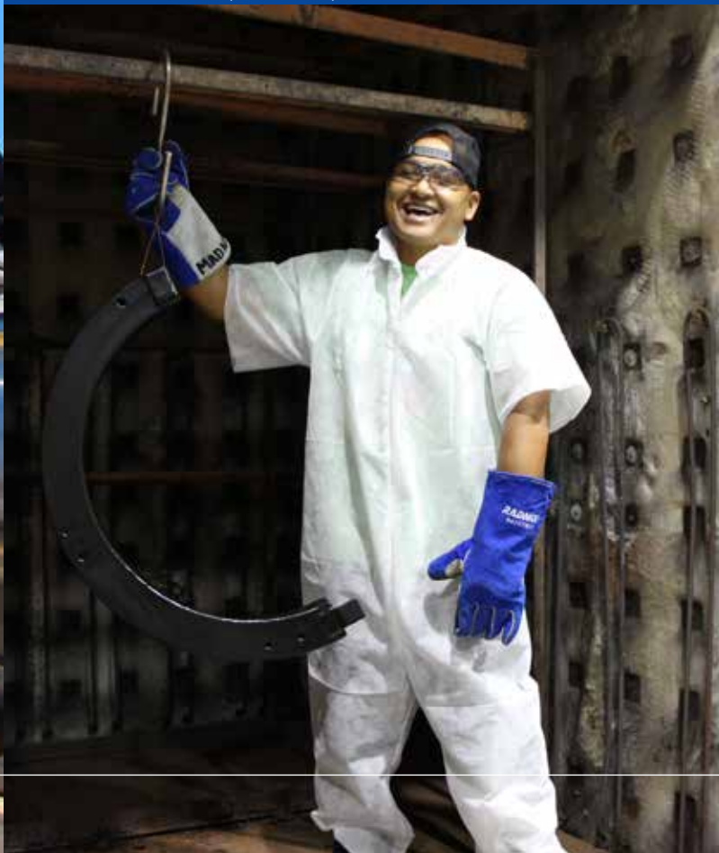
Code 970 Shop 64B Plastic Fabricator Mechanic Mark Corpuz finalizes the baking process on a Hatch Ring coated in Plastisol, in support of USS Columbus (SSN – 762.)
