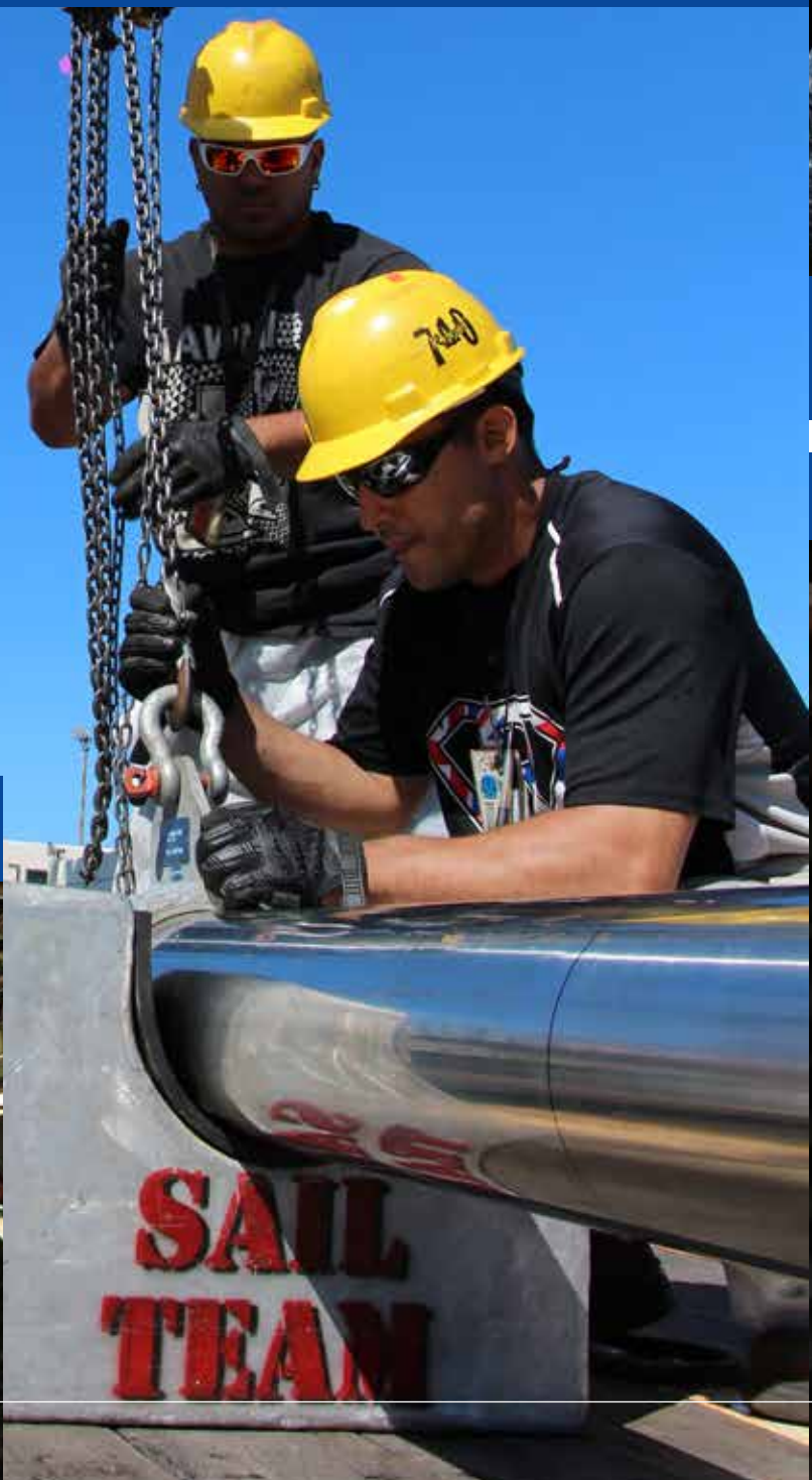
Code 930 Marine Machinist Mechanics Stuart Leong, Ron Gideon and Darren Agena secure metal clamps onto the Periscope in preparation of a crane lift, hoisting it onto the USS Asheville (SSN - 758.)
