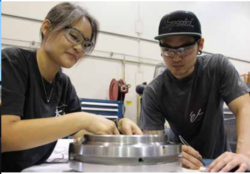
Code 930 Marine Machine Mechanic Contre Gomez, and Marine Machine Mechanic Apprentice Blaze Ravao disassemble a TD – 3 valve, in support of USS Sante Fe (SSN – 763.)
