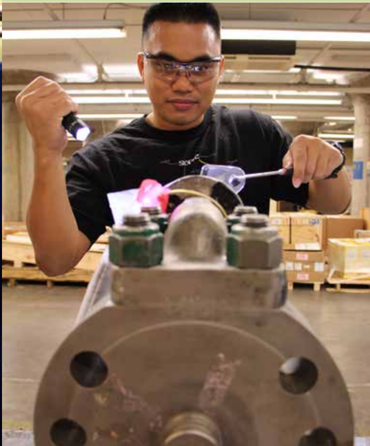
Code 133 Marine Machinery Inspector Leader Ryan Ramiro inspects a submarine safe component in the Non-Nuclear Receipt Inspection area. Code 133 inspects and certifies non-nuclear controlled materials for conformance to technical requirements and end use upon receipt from the supply system or from other activities prior to issue to the projects.
