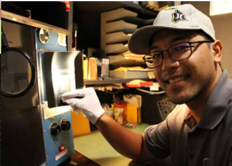
Code 135 Non-Destructive Test Inspector KC Kaleikini interprets radiography film for weld defects.
