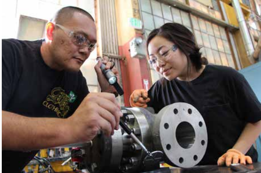
Code 133 Marine Machinery Inspector Leader Chad Ganoot inspects a valve for leakage in the Shop 31 valve section while Shop 31 machinist apprentice Shari Iha looks on. Valves are pressurized and tested on the test stand prior to being considered acceptable for shipboard use.
