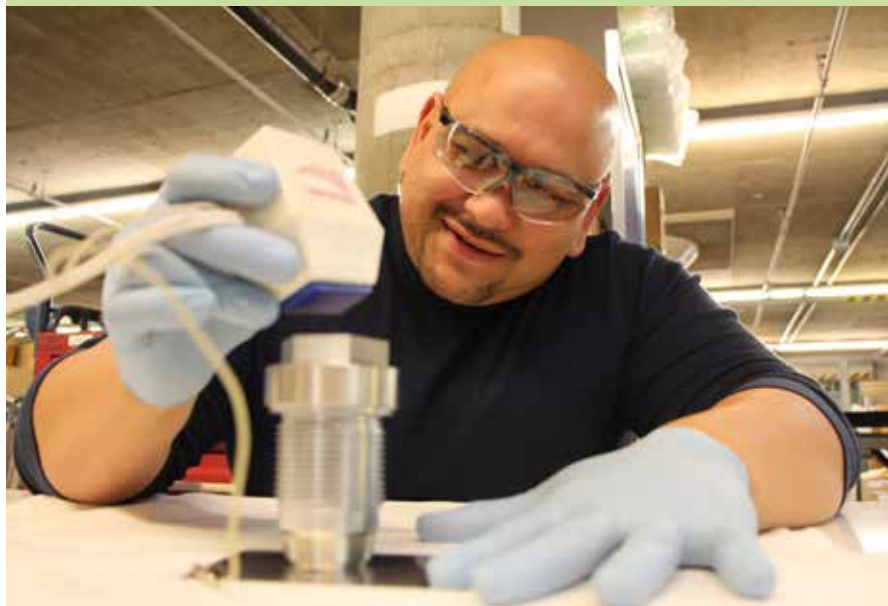
Code 139 Nuclear Inspector Brandon Kaohi performs chemical etching on level 1 material to properly identify the material for traceability.
