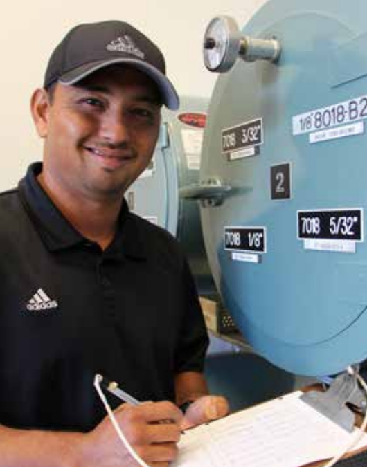
Code 132.2 Quality Assurance Specialist Duane Kuni inspects an electrode oven for filler metal control to ensure proper temperature control.
