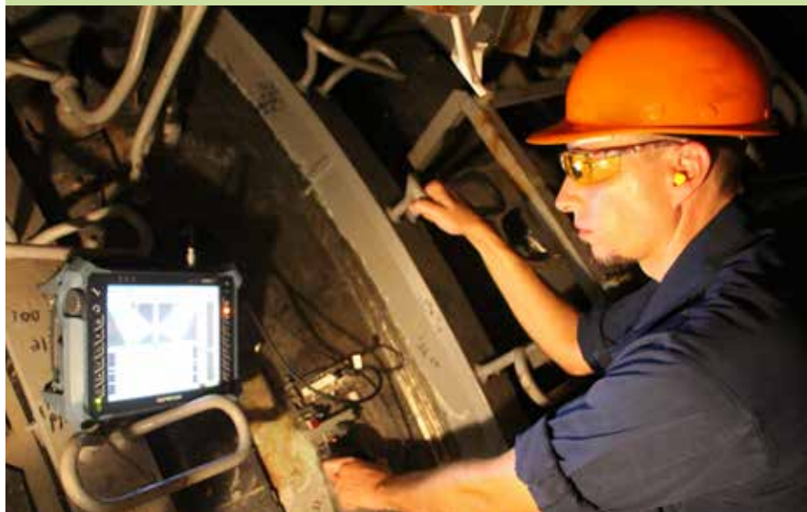
Code 138.3 Lead Ultrasonic Test Examiner Cory Arthur performs a Phased Array Ultrasonic Test on a submarine hull tee weld in conjunction with a monitoring Inspection.
