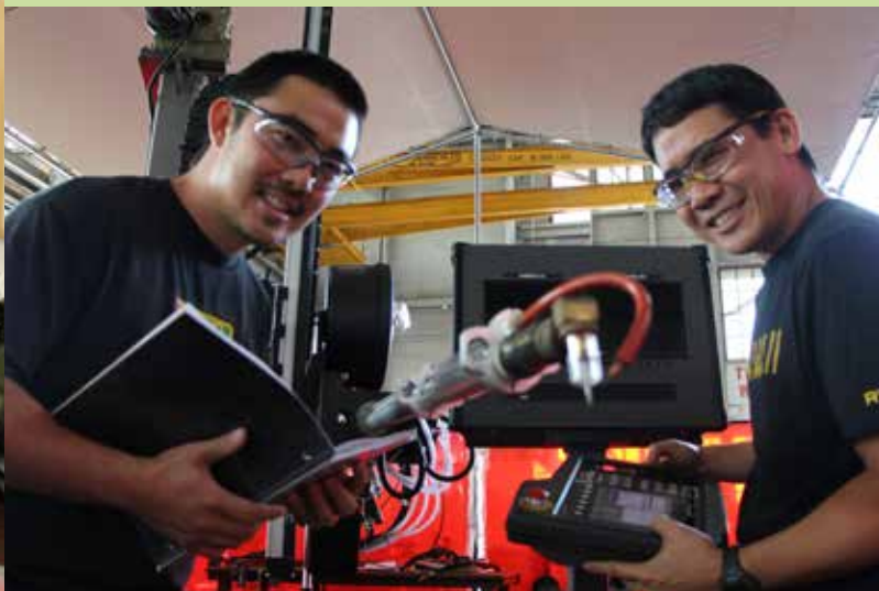
C138 Welding Engineers David Narahara and Craig Mitsui fit check a bore torch that will be used to conduct weld build-ups on shaft couplings using the recently acquired welding machine.
