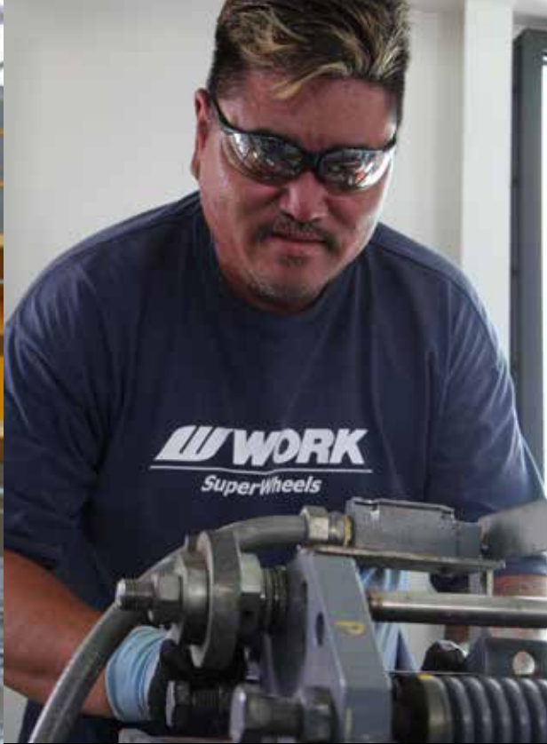
Code 721 Inspector Kevin Achong performs hoist drive train inspections on the main hoist of portal crane P-80.
