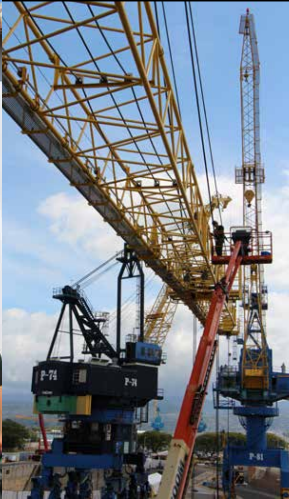
Code 730 Crane Maintenance Mechanic Todd Buhl performing boom maintenance, inspecting structural connections utilizing the 120' area work platform on a Samsung portal crane P-80.
