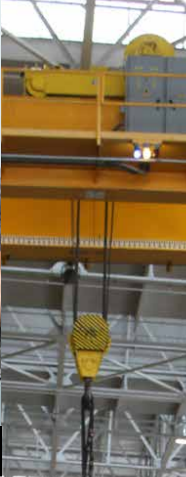
Code 721 Inspector Kevin Achong performs hoist drive train inspections on the main hoist of portal crane P-80.
