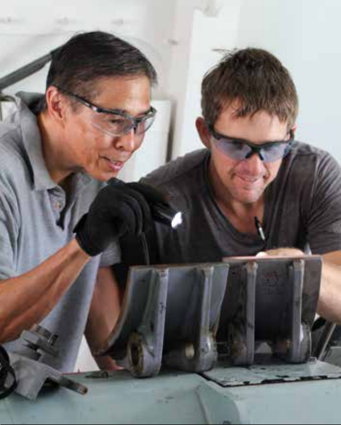
Code 711 Craig Ching and Code 730 Crane Maintenance Mechanic Dave Campbell inspect portal crane brake pads for deficiencies.
