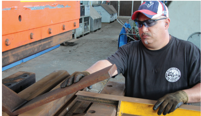
Shop 11 Flange Turner Scott Tom uses "Big Blue" which is the largest of our hydraulic brakes. Flange Turners specialize in the art of shaping metal into complex and intricate shapes for shipboard applications.
