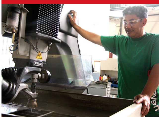
(Below) Shop 11 Shipfitter Jamie Tomisato operates the Flow waterjet. This machine is the workhorse of Shop 11 and has the ability to cut 6" steel with a high level of accuracy. It cuts using a mixture of water and sand grit at pressures over 80,000 psi.
