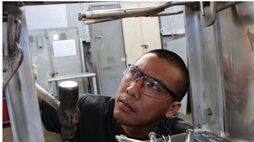
Shop 17 Apprentice Jerry Pagaduan assemble a workbench which will later be installed on the USS Asheville. Shop 17 Sheetmetal personnel specialize in fabricating parts such as lockers, vents, bunks, and trim work out of thin gauge metal.
