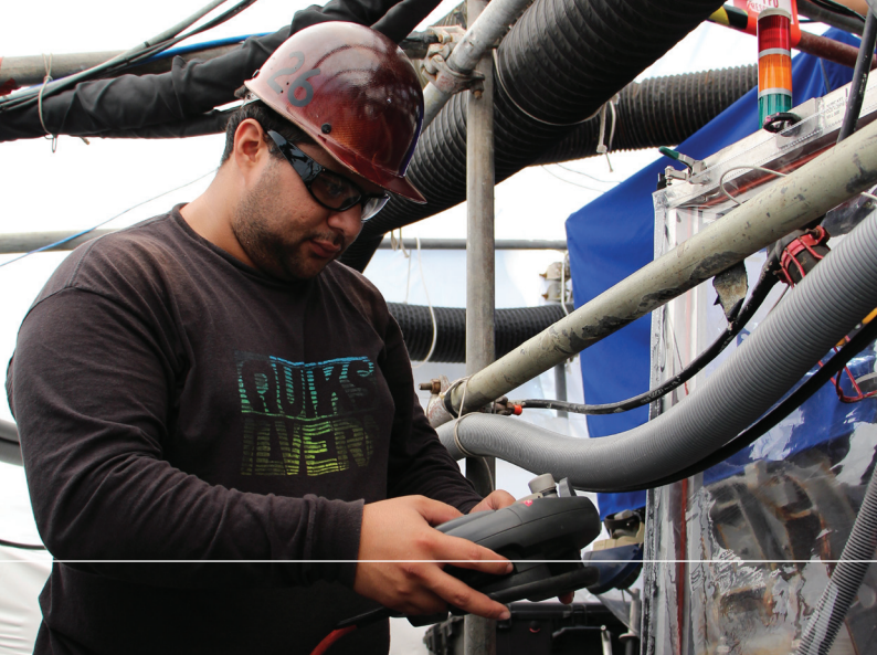
Shop 26 Welder Apprentice Micah Medeiros controls the VLS laser clad welding/grinding machine using a remote pendant. The machine was developed in collaboration with Naval Undersea Warfare Center Keyport and Pennsylvania State University. The laser clad process eliminates brush plating and ultimately restores the gasket sealing area to factory specifications, which ultimately reduces the amount of work on future availabilities.
