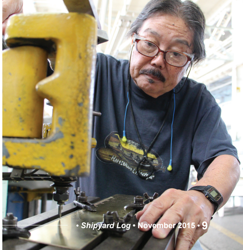
Shop 17 Sheetmetal Mechanic Sydney Higa utilizes the Pantograph Engraver to engrave a stainless steel label plate for one of our submarines. This machine has the ability to engrave on odd shaped materials and components which make this a unique process for Shop 17.
