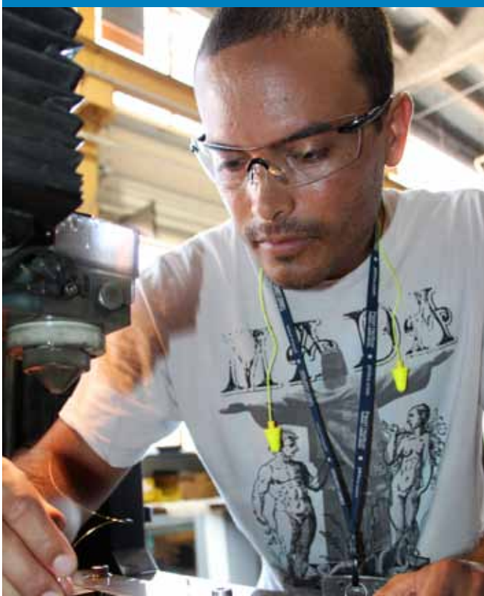
Shop 31 Inside Machinist Brandon Magsayo operates a three-axis vertical mill, while manufacturing a clevis to support operations on a current project.
