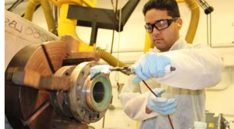
Below: Shop 31 Inside Machinist, first year apprentice, Ryan Jandoc applies a nickel cap on a tailpiece he has mounted on a lathe. The nickel cap is the final coat applied and the final step in the component brushplating process.
