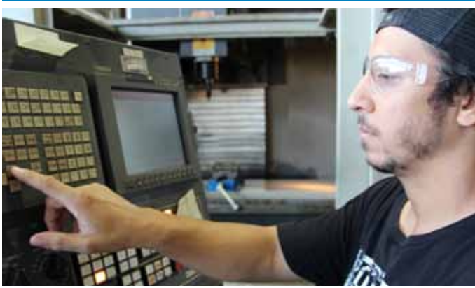
Shop 31 Inside Machinist Brandon Magsayo operates a three-axis vertical mill, while manufacturing a clevis to support operations on a current project.
