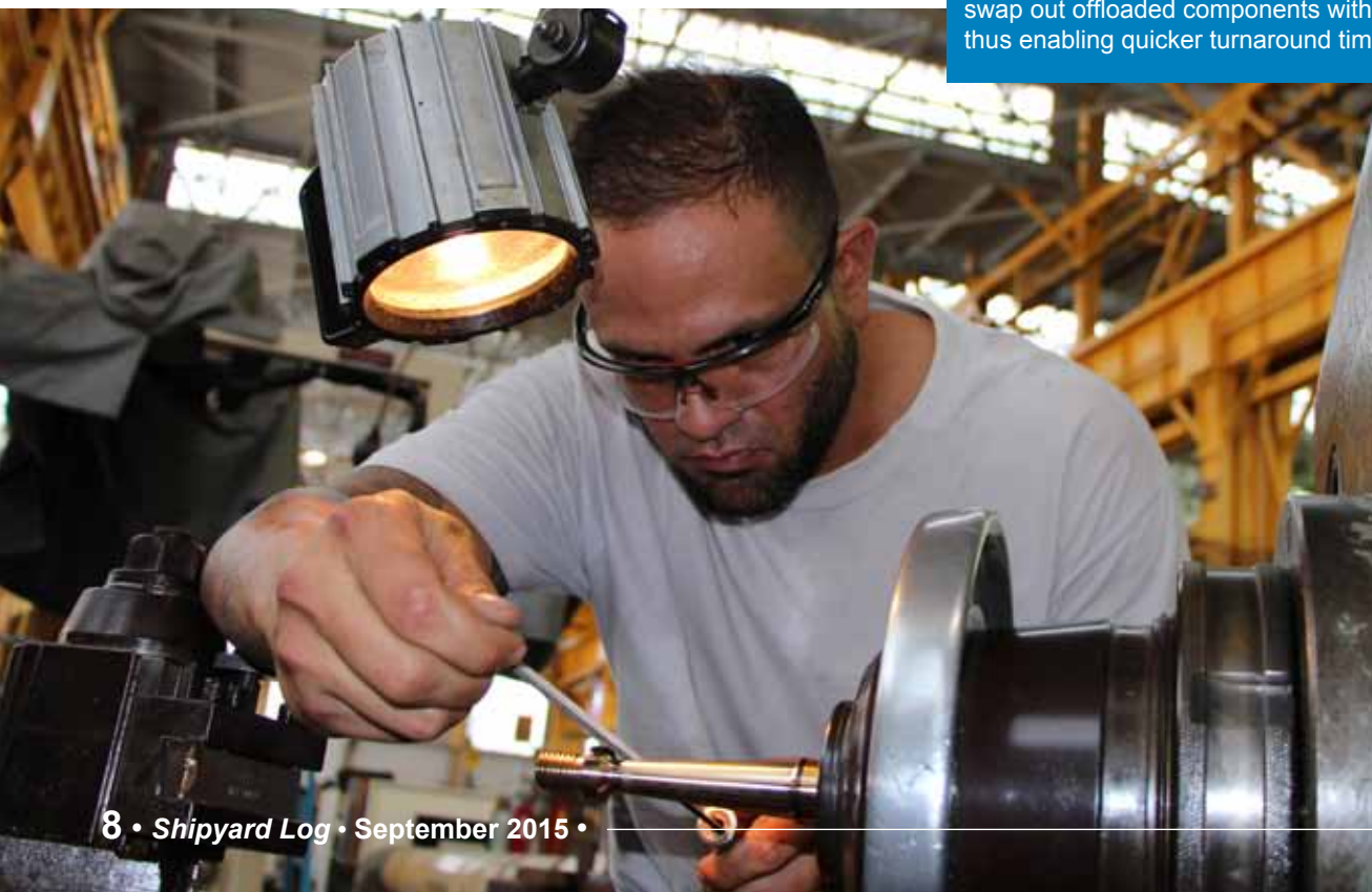
Shop 31 first year Apprentice Machinist Lono Stender works on a manual lathe to improve his practice skills. Lono's work piece will be quality checked for accuracy within the thousandths of an inch by a SME to certify him to work in the M1 machine section
