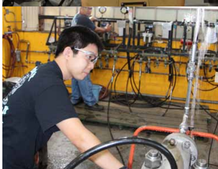
Shop 31 first year apprentices Kevin Maloney (top rear) and Garret Oka prepare for an in-shop test of a hull and backup valve. The valve is a part of the Corporate Component Repair Program, designed to give all future Shipyard availabilities the chance to swap out offloaded components with an "off the shelf" replacement thus enabling quicker turnaround times of repairs.
