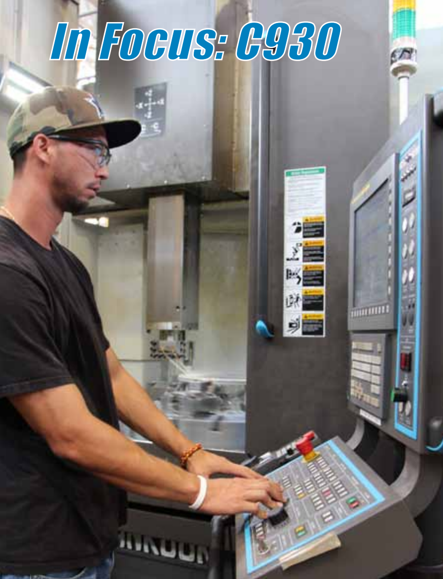
Shop 31 M-1 Elite Mechanic Spenser McCready performs a multi-axis cut on a state-of-the-art, Hanlock vertical turret lathe to manufacture a shim for the sonar dome.
