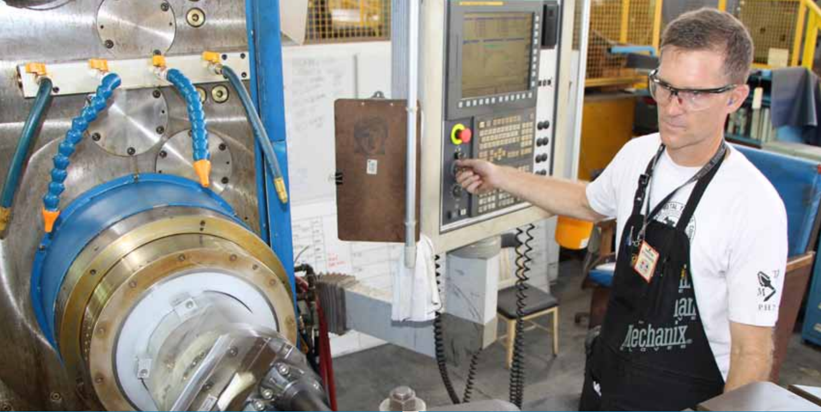
Above: Shop 31 Inside Machinist Doug White uses the Giddings and Lewis PT1800 CNC 5 axis horizontal machining center to prep a pipe elbow for welding with its contouring head attachment. The versatile machine enables the shop to support many critical machining operations, which has reduced execution time.
