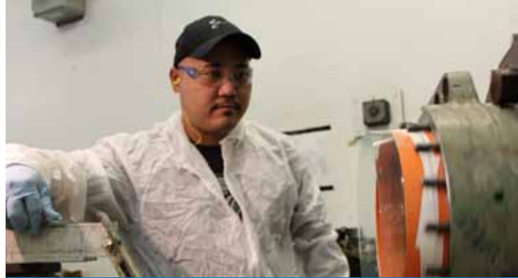
Shop 31 Inside Machinist brushplating Subject Matter Expert (SME), Reid Nagamine is watching to ensure this housing component is being plated with nickel correctly. The housing will be routed to Shop 31's grinding section where it will be ground to size.
