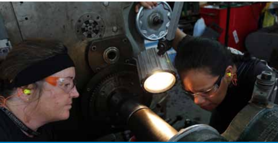
Shop 31 Inside Machinist Apprentice Tabby Lynn-Stakes works with Inside Machinist Mechanic Tamia Keolanui during a complex line-boring operation. Line-boring is used to machine internal surfaces concentric to each other. It involves a complex setup and specialized training since most cuts are performed where there is little to no visibility.
