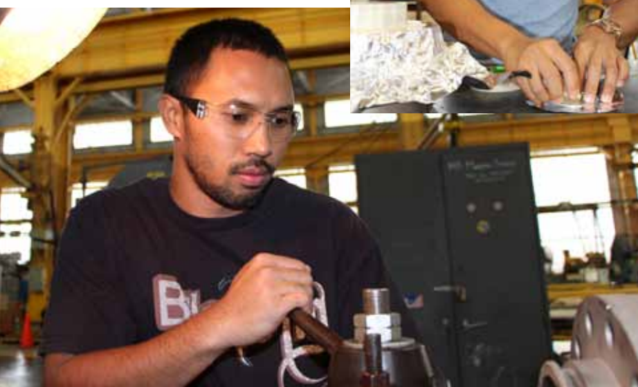
Shop 31 Valve Mechanic Blake Furtado exercises his machinist skills to perform minor machining operations on a valve tailpiece. Blake's addition to the valve team has helped inspire the installation of a lathe and small mill in the valve section. He has almost singlehandedly allowed the valve section to decrease turnaround times and increase throughput.
