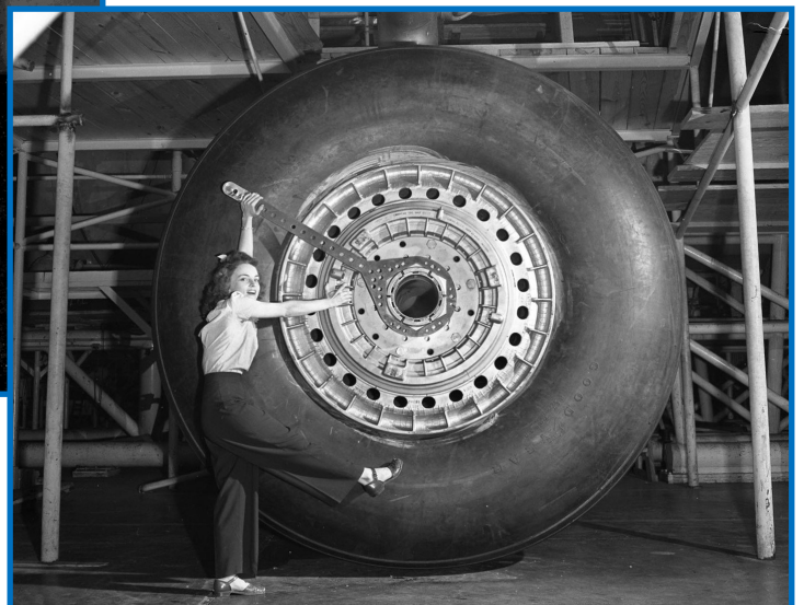
Left: Maurine Fisher of Goodyear holds the popular 6.00 x 6" wheel that is standard on light aircraft. The 110-inch wheel she is sitting on weighs over 4,000 pounds with tire, tube and brake, while the smaller unit weighs 15 pounds complete.
