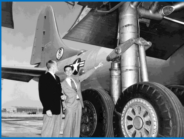
Top: Convair executives examine the main landing gear of the B-36 Peacemaker .
