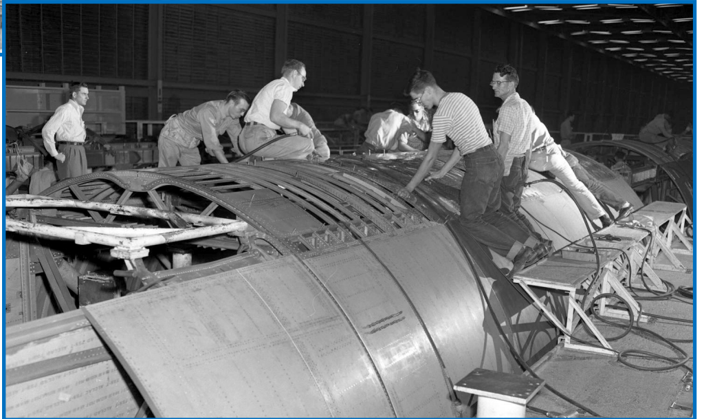
Above: Due to the size of some structures on the B-36, these areas required numerous technicians working together on a single assembly area such as the bomb bay structure shown here.
