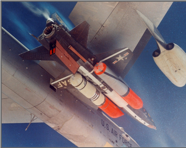
The X-15A-2 with external propellant tanks installed prepares for launch at the beginning of flight 2-45-81 on 1 July 1966 (AFFTC/HO photo)
