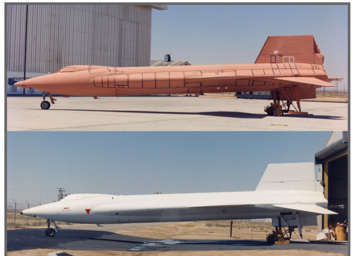
The Martin Marietta MA-25S ablative applied to the X-15A-2 was pink in color and utilized a white sealer coat to protect it from the liquid oxygen propellant (NASA photo).
