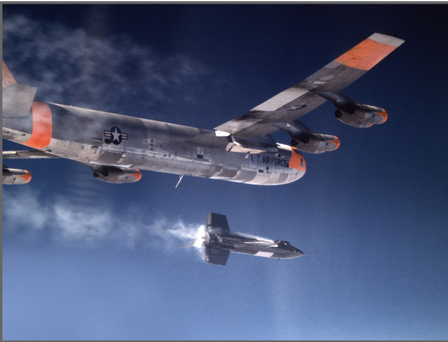
X-15 Ship 2 is launched on an early contractor flight using the interim XLR11 engines (North American Aviation photo)
