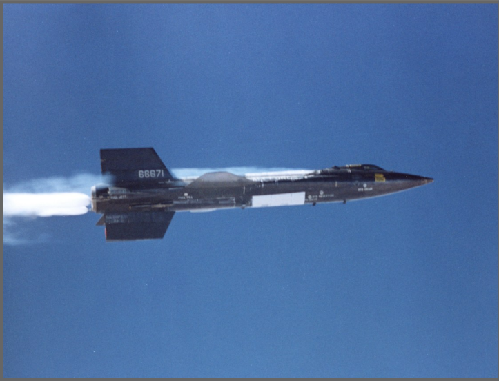
The beginning of X-15 flight 2-28-48 on 29 August 1962 took Maj Rushworth to a speed of Mach 5.12 (3,447 mph) and an altitude of 97,200 feet (AFFTC/HO photo)
