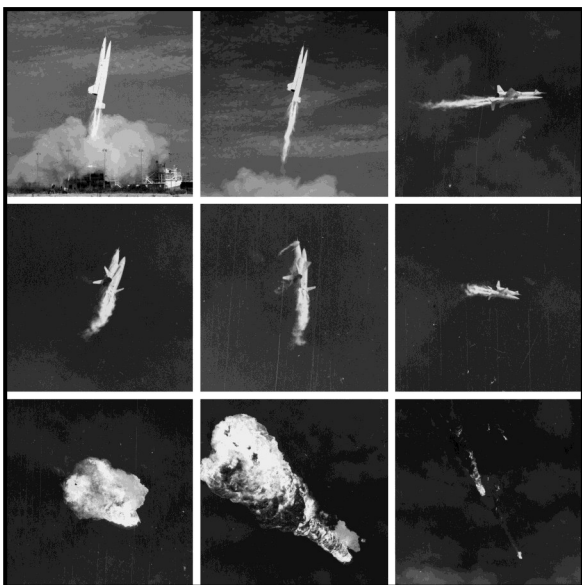
The first XSM-64 Navaho launch experienced severe pitch oscillations early in its flight before it broke up after reaching an altitude of only 10,000 ft
