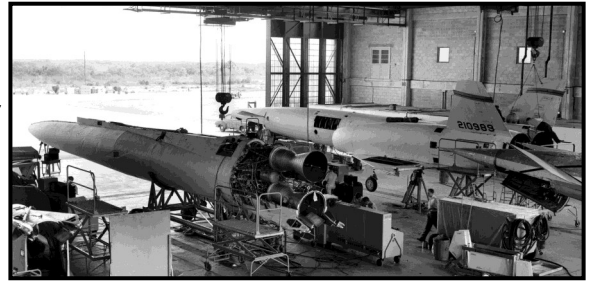
The first XSM-64 launched, sits in its hangar at the East Coast launch facility undergoing final assembly and testing. Clearly seen are the Rocketdyne XLR71 engines on the booster.
